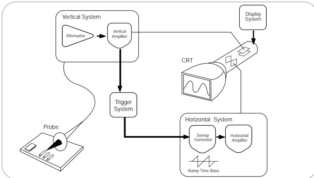
► **Figure 13.** The architecture of an analog oscilloscope.
