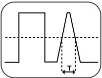
**Glitch Triggering.** Glitch triggering allows you to trigger on digital pulses when they are shorter or longer than a user-defined time limit. This trigger control enables you to examine the causes of even rare glitches and their effects on other signals
