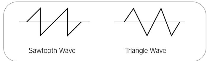
▶ **Figure 7.** Sawtooth and triangle waves.
