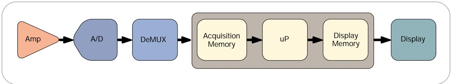
▶ **Figure 16.** The serial-processing architecture of a digital storage oscilloscope (DSO).
