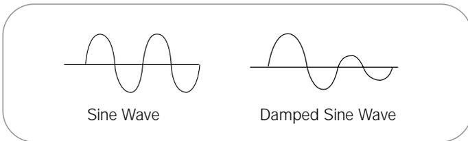
▶ **Figure 5.** Sine and damped sine waves.
