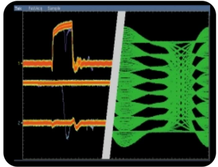
► **Figure 19.** Some DPOs can acquire millions of waveforms in just seconds, significantly increasing the probability of capturing intermittent and elusive events and revealing dynamic signal behavior.
