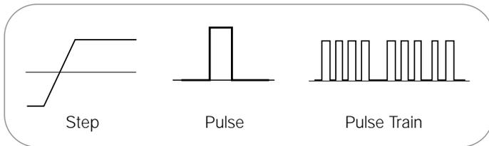
► **Figure 8.** Step, pulse and pulse train shapes.
