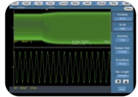
► **Figure 53.** Capturing the high frequency detail of this modulated 85 MHz carrier requires high resolution sampling (100 ps). Seeing the signal's complete modulation envelope requires a long time duration (1 ms). Using long record length (10 MB), the oscilloscope can display both.
