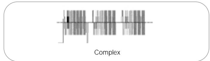
► **Figure 9.** An NTSC composite video signal is an example of a complex wave.
