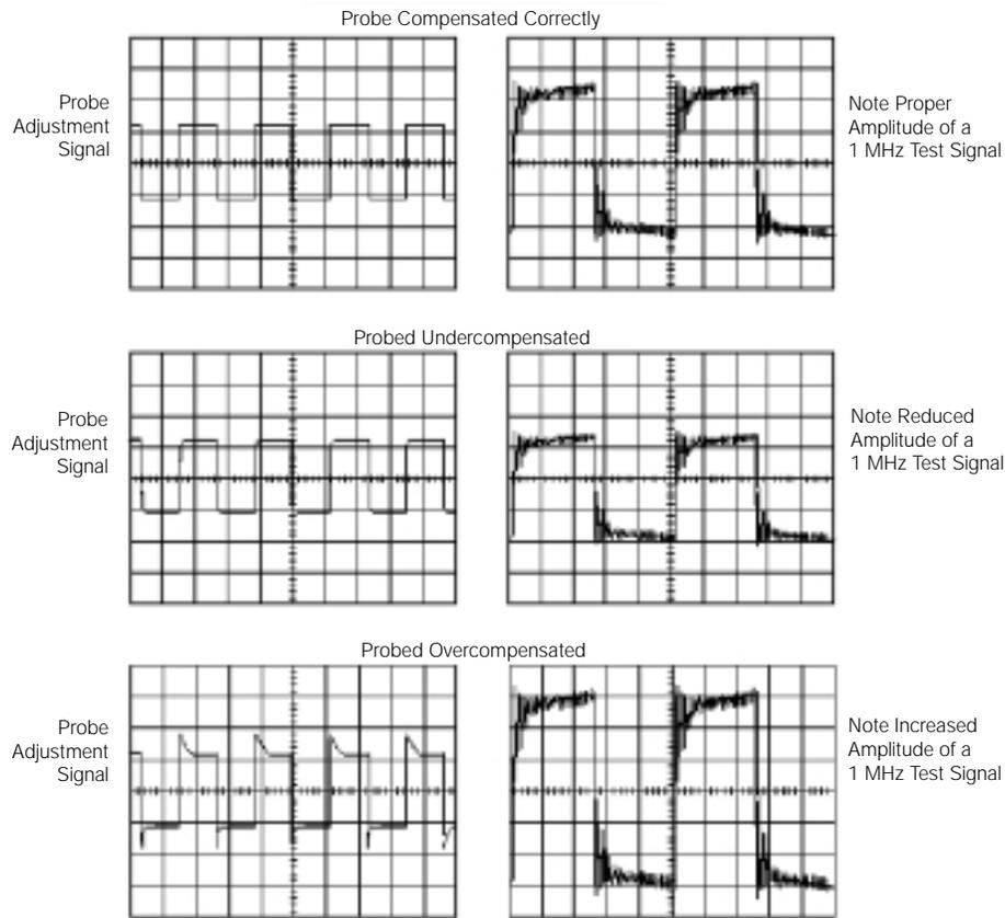
▶ **Figure 65.** The effects of improper probe compensation.
