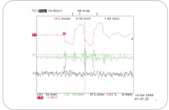
▶ **Figure 43.** Differential probes can separate common-mode noise from the signal content of interest in today's fast, low-voltage applications – especially important as digital signals continue to fall below typical noise thresholds found in integrated circuits.
