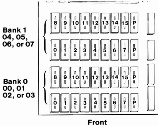
Figure 3. Type 1 System Board Memory
