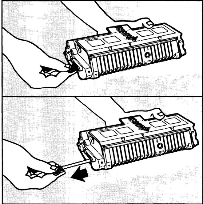
Figure 7-5. Removing the Sealing Tape
