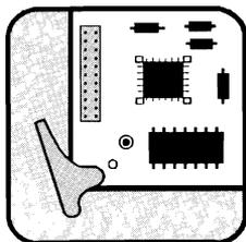
Installation of the HP 33474B one-megabyte or HP 33475B two-megabyte RAM memory board allows you to expand the HP LaserJet IIIP printer's standard memory by an additional four megabytes. There are two memory expansion slots. You can install any combination of one- or two-megabyte boards. Four megabytes is the maximum expanded memory the printer can use.
