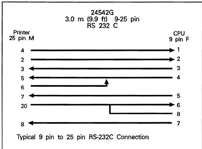
**Figure D-2. Typical AT Pin Assignments**
