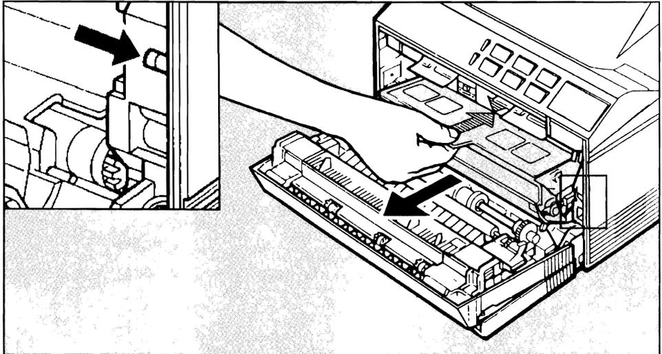
**Figure 7-2. Removing the Used Cartridge**
