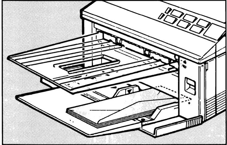
Figure 3-8. Inserting an Envelope into Manual Feed Tray
