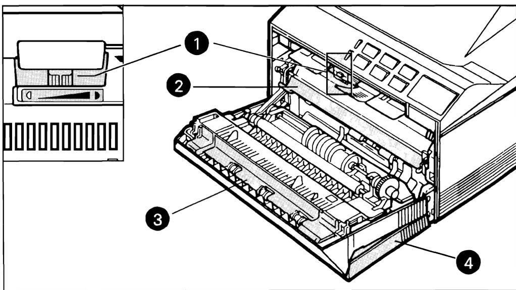
Figure 1-6. Inside the Paper Path Door
