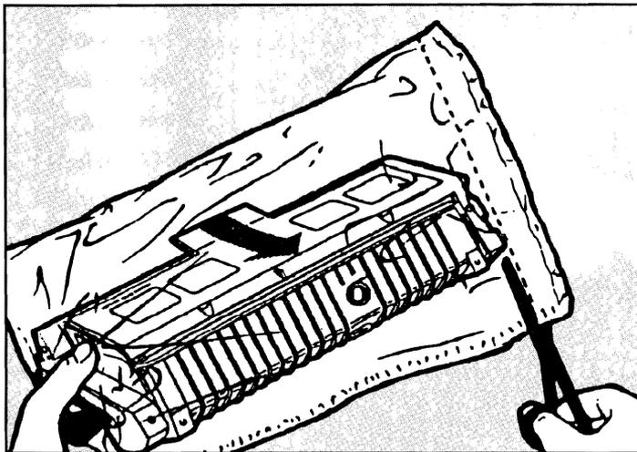
Figure 7-3. Removing the Toner Cartridge
