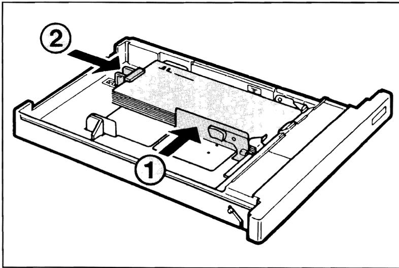
Figure 4-11. Adjusting the Width and Length Guides
