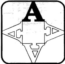
Whether or not the original font is in the orientation or print direction you want, the HP LaserJet IIIP printer can automatically rotate type in 90° increments. Figure 6-12 shows a single portrait font automatically rotated using the print direction command.
