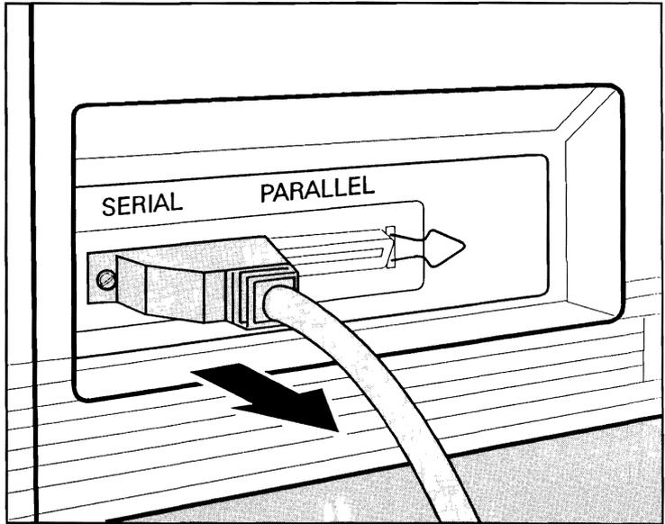
**Figure D-4. Disconnecting Cord and Cable**
