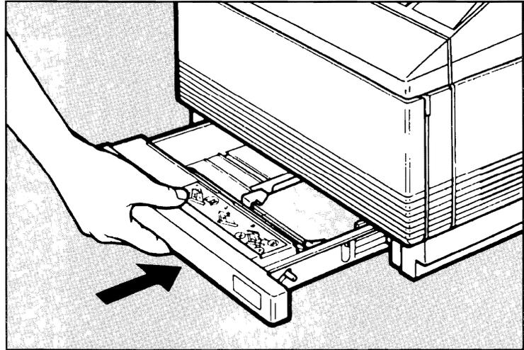
Figure 4-12. Installing the Envelope Tray
