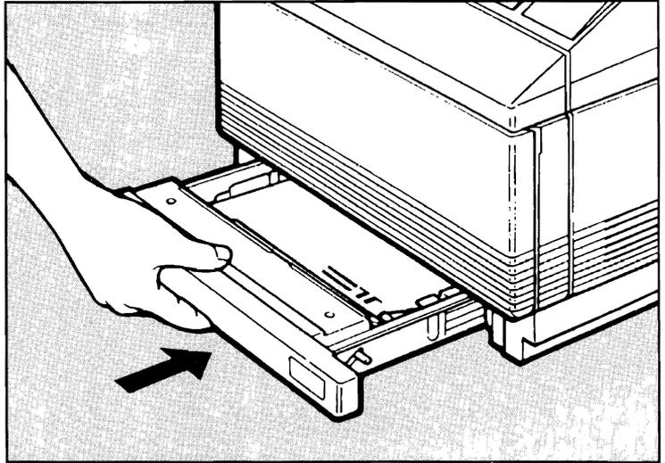
Figure 4-5. Inserting the Tray
