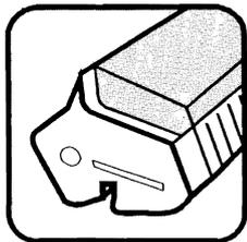
The toner (EP-L) cartridge in your Hewlett-Packard HP LaserJet IIP printer has been designed to simplify the replacement of your printer's "consumable" items. The toner cartridge contains a print drum and a supply of toner.
