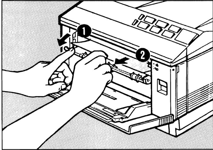
**Figure 8-7. Clearing the External Fuser Access Door**
