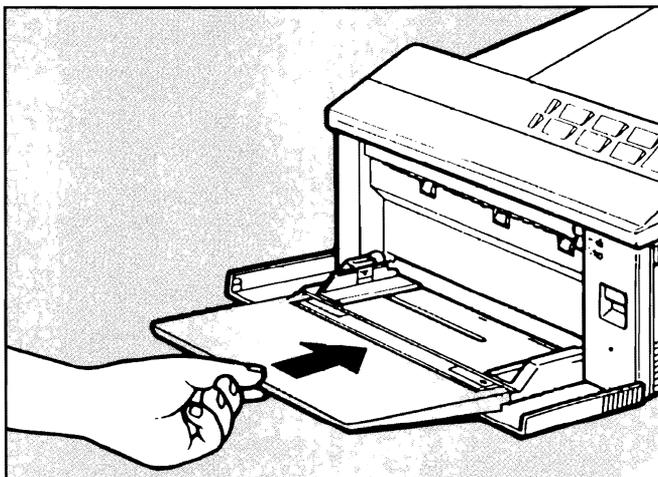
Figure 3-2. Attaching the Enhanced MP Tray Extender
