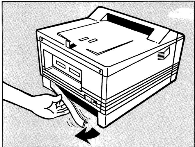
Figure 4-7. Removing the Flap
