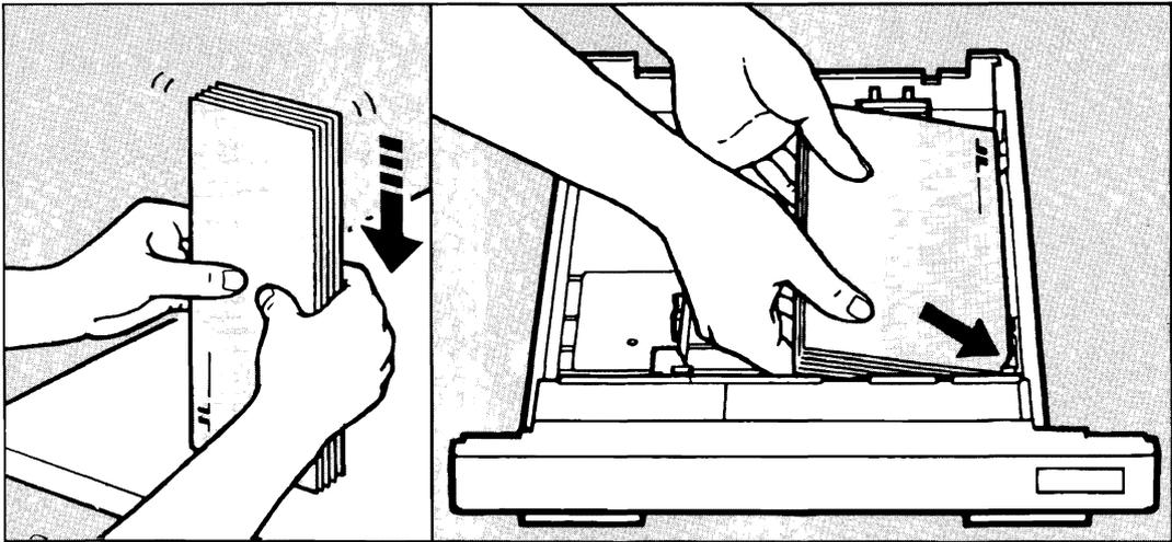
Figure 4-10. Placing the Envelope Stack in the Tray
