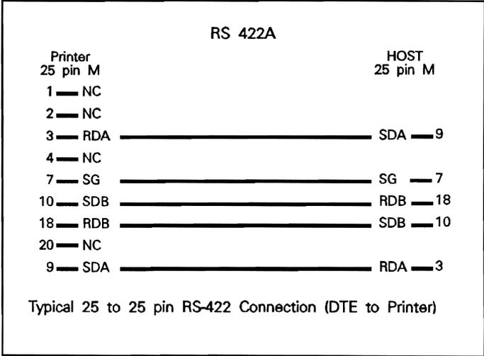
**Figure D-3. Typical RS-422A 25-25 Pin Assignments**
