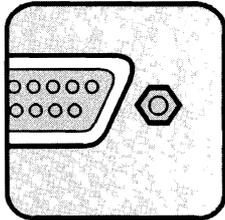
Use a serial interface when you need to locate the printer far away from your computer (up to 15.5 meters). Serial interfaces are not as fast as parallel.
