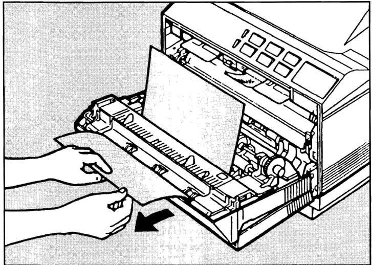
Figure 8-5. Clearing a Paper Jam in the Fuser Roller Area
