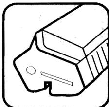
When the toner supply in the toner (EP-L) cartridge gets low, some parts of a page may exhibit light printing or no printing at all. You can often extend the life of the cartridge by up to 50 pages by redistributing the remaining toner in the toner cartridge.
