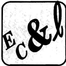
PCL printer commands always begin with the escape character ( $E_C$ ). The escape character precedes a unique series of letters and numbers that tell the printer what to do (see figure 5-4). Software packages have different ways of inserting or representing  $E_C$ , most commonly by its numeric character value: 27 in decimal or 1B in hexadecimal.
