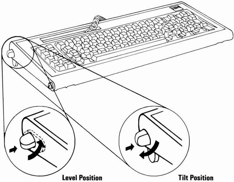
To attach the keyboard to the front panel press the adjustable leg handles in and slide them into the bottom holes on the system unit's front panel.
