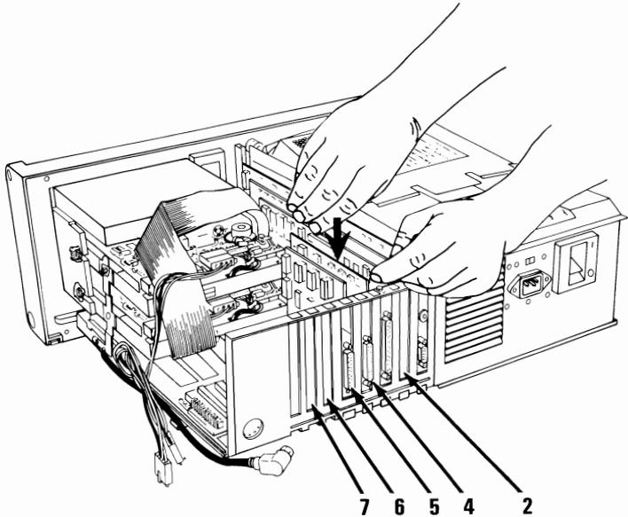
**67** Align the slot of the option retaining bracket with the threaded screw hole in the rear panel of the system unit.
