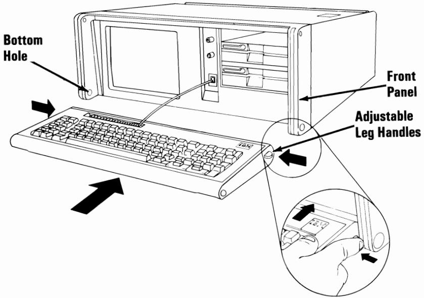
When the keyboard is attached to the front panel it may be placed in the stored position.
