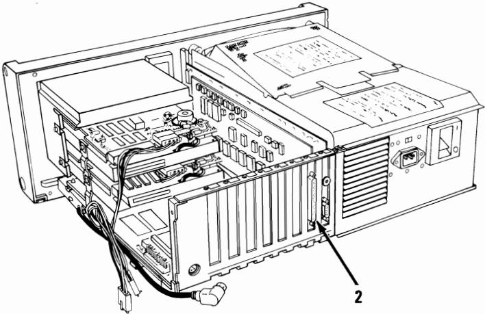
**57** Connect the Diskette Drive Signal Cable to the front end of your Diskette Drive Adapter as shown below.
