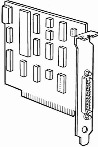
This option consists of the Asynchronous Communications Adapter. If it is missing or damaged, notify your place of purchase.
