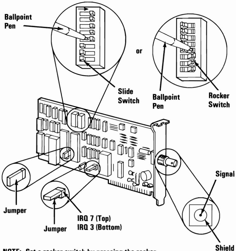
**NOTE:** Set a rocker switch by pressing the rocker down to the desired position.
