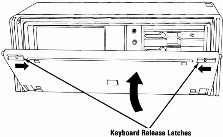
To lower the keyboard down to the operating position, press the two keyboard release latches toward the center of the system and lower the keyboard. Release the latches.
