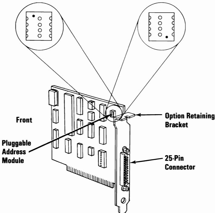
**2** The possible interfaces for the Asynchronous Communications Adapter are the current-loop and RS232-C. Arrange the pluggable module for the interface that suits your application, as shown in the figure below.
