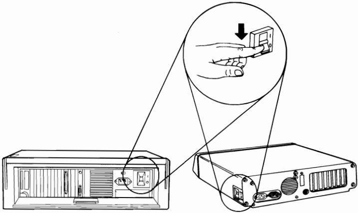
**8** Unplug the system unit's and expansion unit's power cord from the wall outlet. Disconnect all cables and power cords from the rear of the units.
