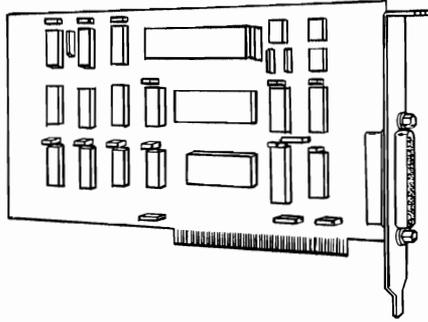
This option consists of the Binary Synchronous Communications Adapter. If it is missing or damaged, notify your place of purchase.
