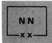
Stations that have the Power switch set to On are displayed in reverse video, and their boxes are marked by two X's.
