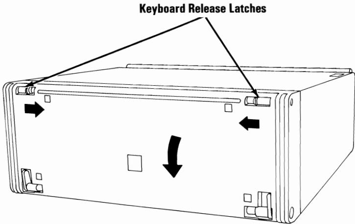
To separate the keyboard from the front panel, push in on the adjustable leg handles by putting a finger in each of the front panel's bottom holes. Pull the keyboard away from the front panel.
