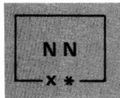
If another Personal Computer has the same station address as your Personal Computer, a long beep will sound every 3 seconds, the box will be displayed in blinking reverse video and marked by an X and an asterisk.
