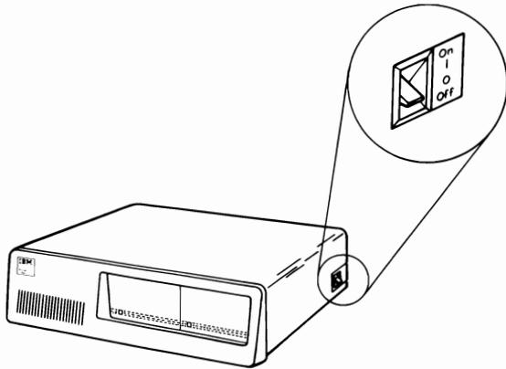
The expansion unit has only one control -- the Power switch. Whenever power is to be applied to the IBM Portable Personal Computer, the Power switch on the expansion unit must be set to On first. If this is not done, an error message appears on the display. To recover, set the Power switches on both the system unit and expansion unit to Off. Set the Power switch on the expansion unit to On first, then the Power switch on the system unit.
