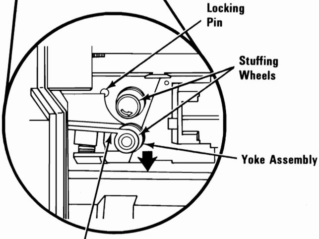
**Pull the Yoke Assembly here**
