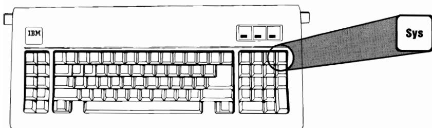
The Print Screen (PrtSc) key when pressed displays an asterisk (\*). If you press and hold a shift key and then press Print Screen (PrtSc) most programs will print (if you have a printer) the data that is displayed on your screen.
