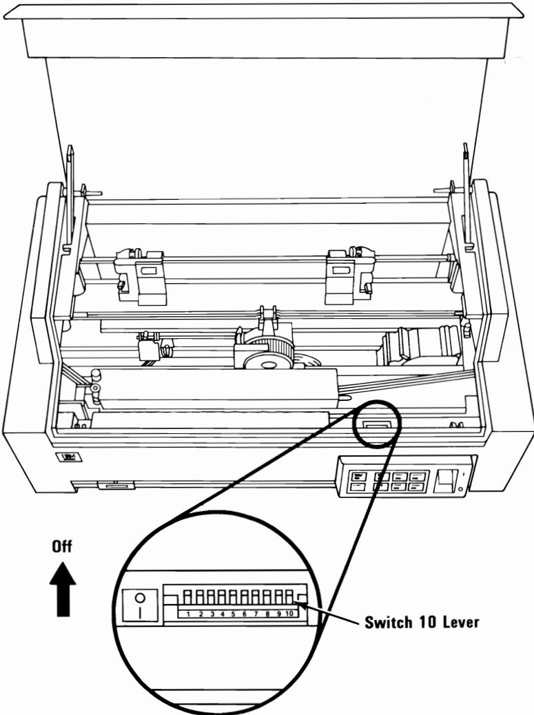
By turning DIP (Dual In-line Package) switches 9 and 10 off, you will get the same printout each time you run the printer self-test. If the printout does not print correctly, your printer may require service.
