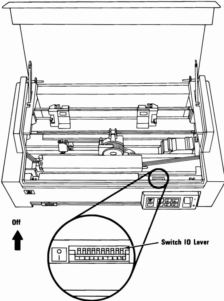
By setting DIP (Dual In-line Package) switches 9 and 10 off, you will get the same printout each time you run the printer self-test. If the printout does not print correctly, your printer may require service.
