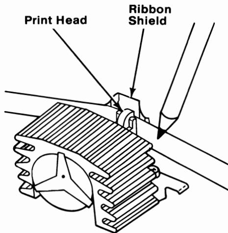
**9** Turn the knob in the direction of the arrow to remove any slack in the ribbon.
