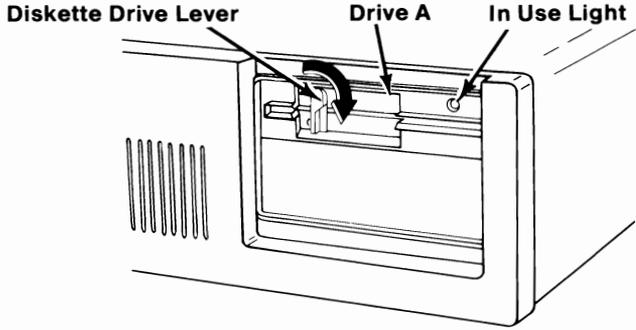
When the in-use light is on it indicates that your system unit is using your diskette drive.
