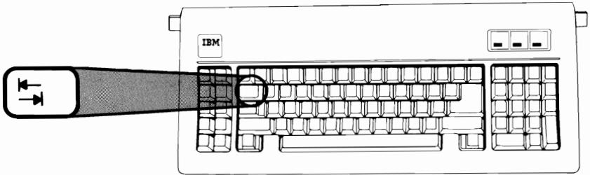
There are two Shift keys on your keyboard. Pressing either of the Shift keys switches the letter keys, the symbol keys and the numeric keypad keys from Lower case mode to the Upper case mode.
