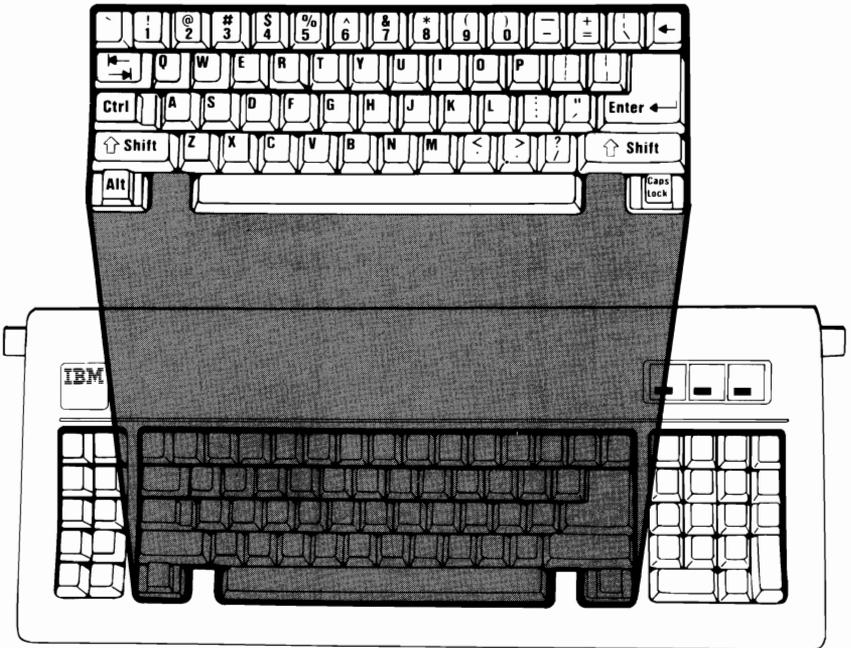
The Enter key works like a carriage return by moving the cursor to the start of a new line. The Enter key is often used to tell your IBM Personal Computer AT to start doing a job.
