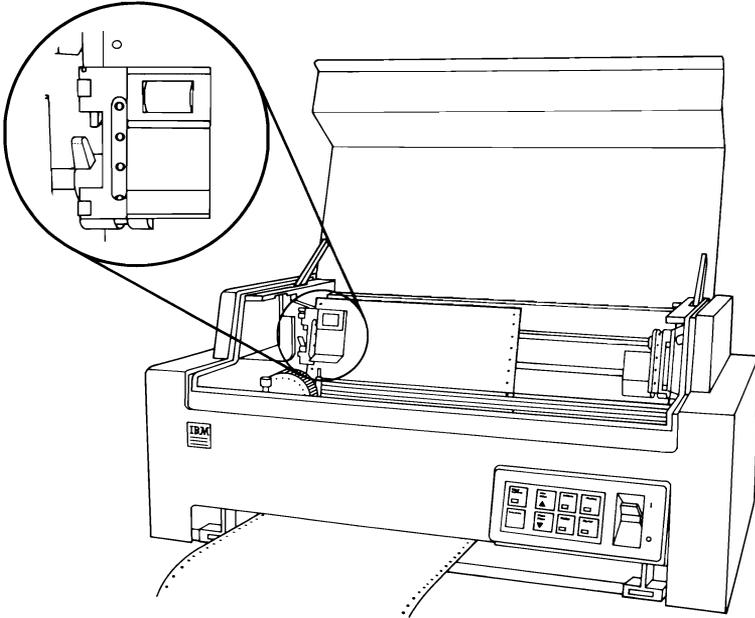
**15** Adjust the right tractor so the tractor pins align with the holes in the right side of the paper.
