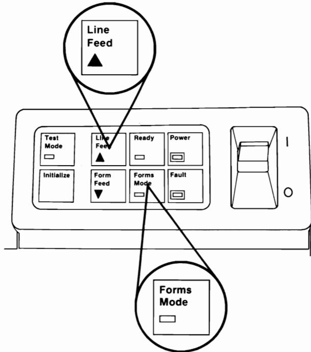
**14** Watch the paper and press the Form Feed button. The paper moves down 0.176 mm (1/144 in.). Notice that this button works differently when the printer is in the forms mode.
