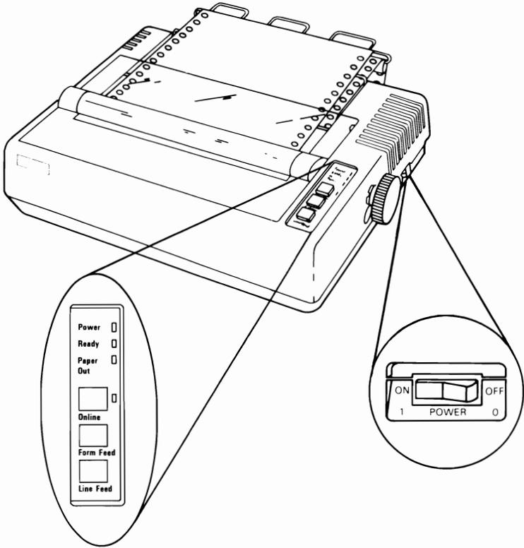
**POWER** When the printer's power is on the power light on the control panel will come on.
