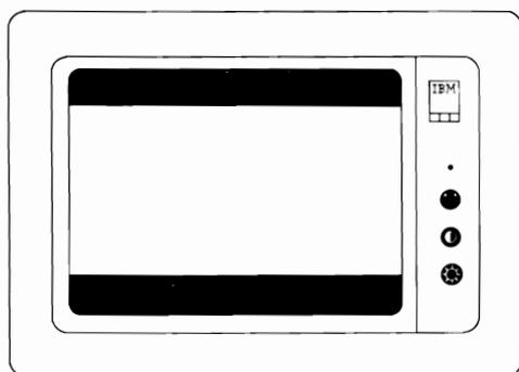
**6** Turn the Vertical Size control clockwise until the black area at the top and bottom of the screen just disappears. If one of the black areas disappears before the other, continue to turn the Vertical Size control until the second black area is gone.
