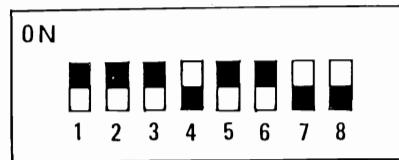
2. Your PC has 128K RAM installed on the motherboard. Insert 512K of additional RAM on your MEMO576 RAM card, to reach the maximum capacity of DOS. (640K) Your DIP switch settings will be:
