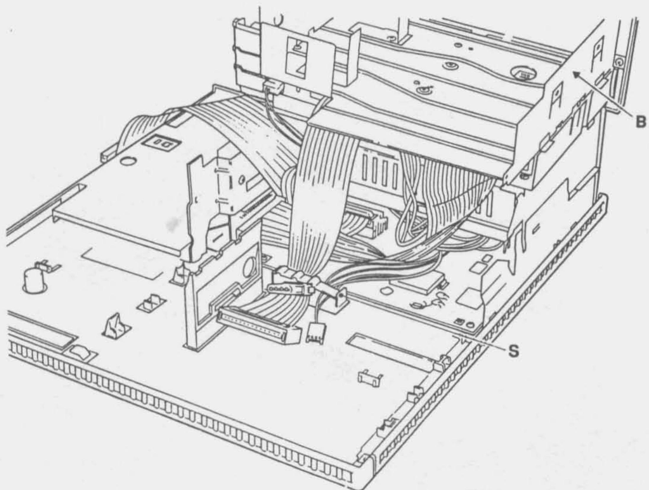
8) Re-place the drive support unit B to its position.
