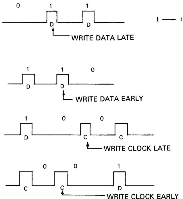
Writing should occur out of a shift register which is used to observe the pattern. "On time" represents a nominal delay. Early and late represent less and more delay respectively.
