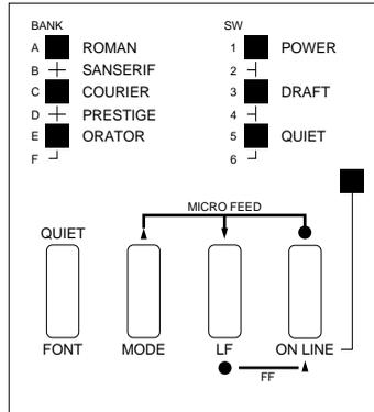
This chapter describes general functions that can be performed using the control panel buttons while the printer is turned on and either on-line or off-line. The buttons perform different functions in the EDS and Dot Adjustment Modes. Functions of control panel buttons in these modes are described in the relevant sections covering them.
