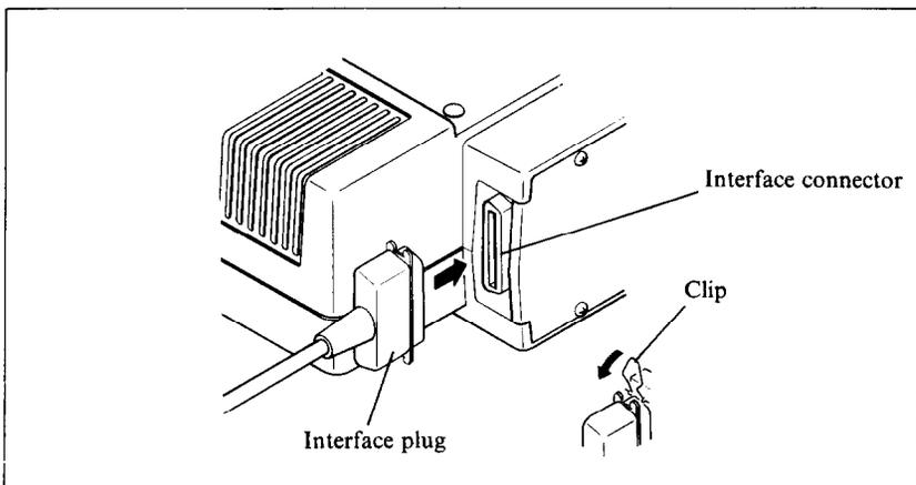
**Figure 3-1.** SD-10/15 has parallel interface as standard.
