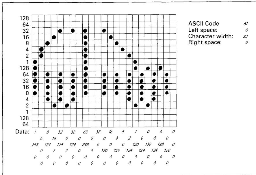
Figure 8-5. Add the values of the dots into three bytes.
