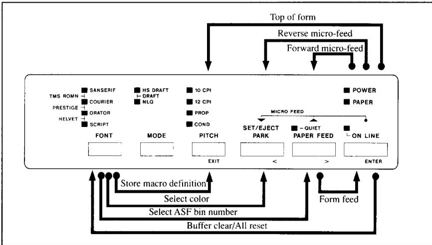
Figure 5-7. Switch combination functions of control panel.
