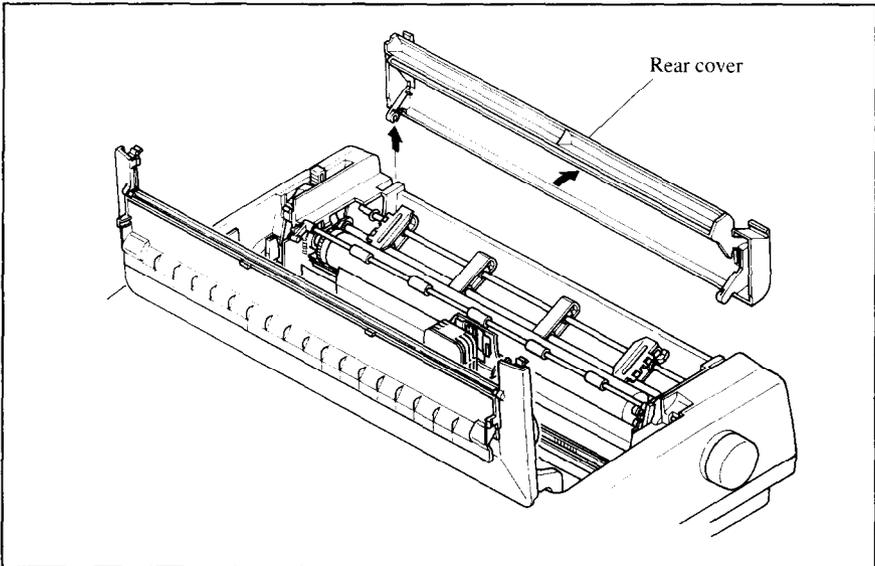
**Figure 3-2.** Open the rear cover, and remove it.
