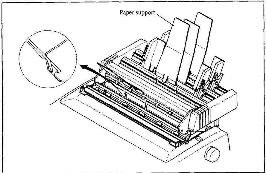
**Figure 3-8.** Attach the clear plastic paper supports to the Automatic Sheet Feeder.
