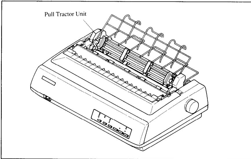
**Figure 4-6.** Install the optional Pull Tractor Unit.
