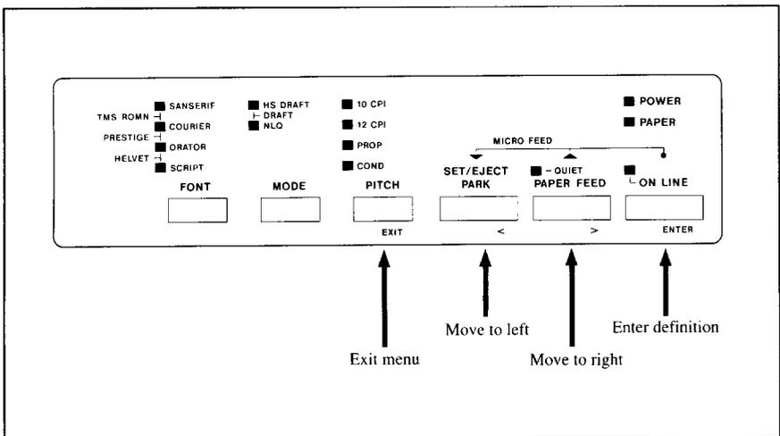
Figure 6-1. Button functions in the Memory Switch mode.
