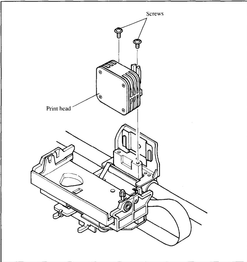
**Figure 10-1.** Replacing the print head.
