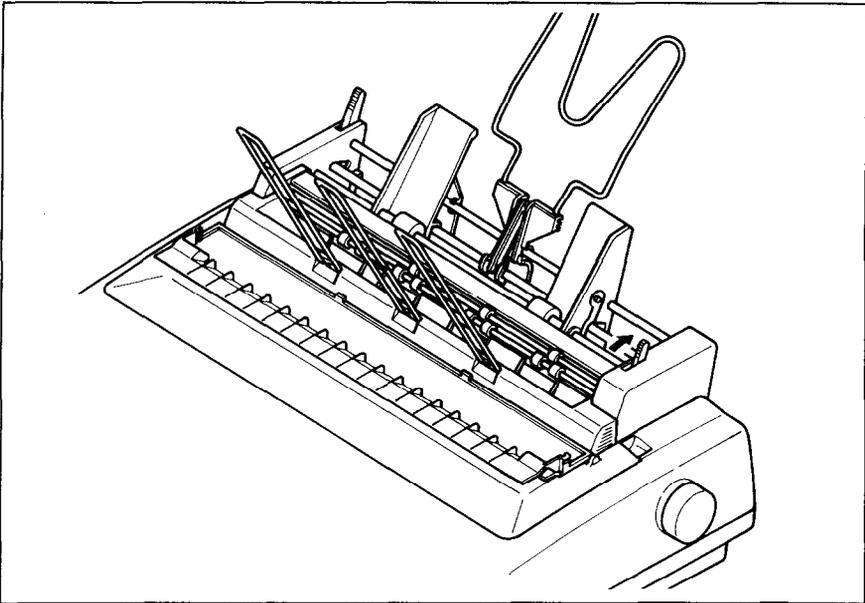
**Figure 4-14.** Install the optional Automatic Sheet Feeder.
