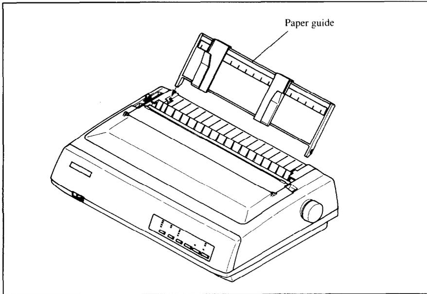
**Figure 4-12.** Mounting the paper guide for single sheets.
