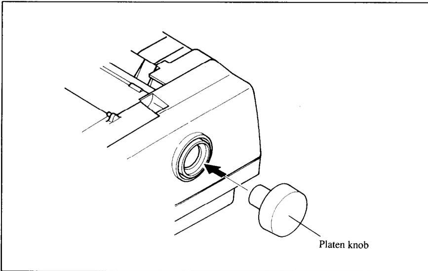
**Figure 2-2.** Mount the platen knob.
