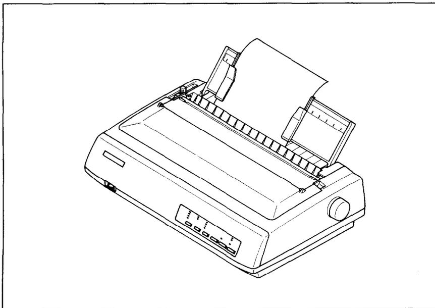
*Figure 4-13.* Loading a single sheet.
