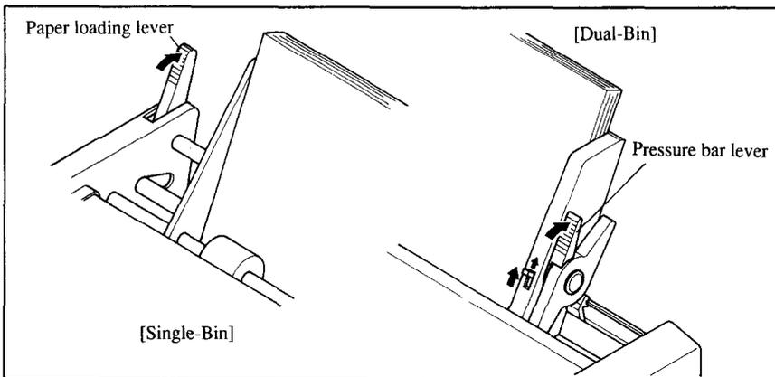
**Figure 4-18.** Push the paper loading lever or pressure bar levers to hold the paper stack.
