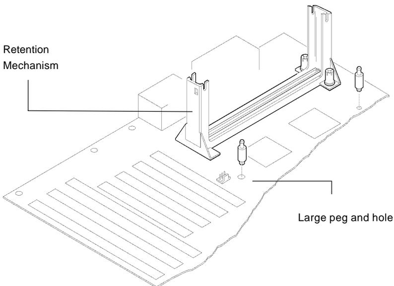
3. Slide a black plastic support onto each end of the fan/heat sink making sure that the hole and clip are on the outside edge of the support. If the supports are reversed, the holes will not line up with the pegs on the motherboard. Slide each support toward the center of the processor until the support is seated in the outside groove in the fan housing.
