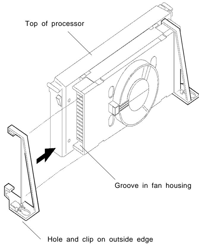
4. Slid the clip (A) on each support toward the processor, exposing the hole that will fit over the peg on the motherboard. Push the latches (B) on the processor toward the center of the processor until they click into place.
