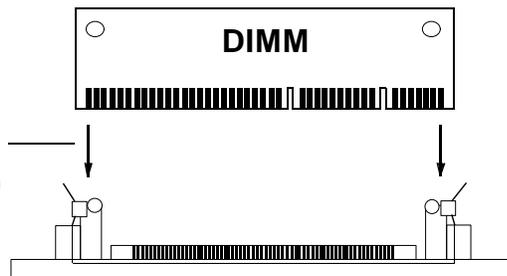
**Figure 2-7. Installing/Removing a DIMM Memory Module**
