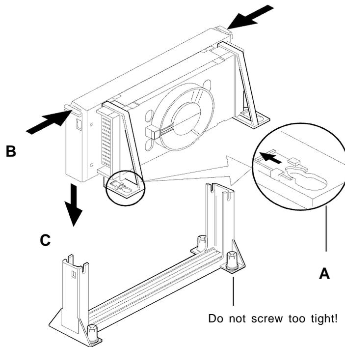
6. Slide the clips on the supports (A) forward until they click into place to hold the pegs securely. Apply slight pressure on the peg and push the peg toward the clip while pushing the clip forward. Push the latches on the processor (B) outward until they click into place in the retention mechanism. The latches must be secured for proper electrical connection of the processor.
