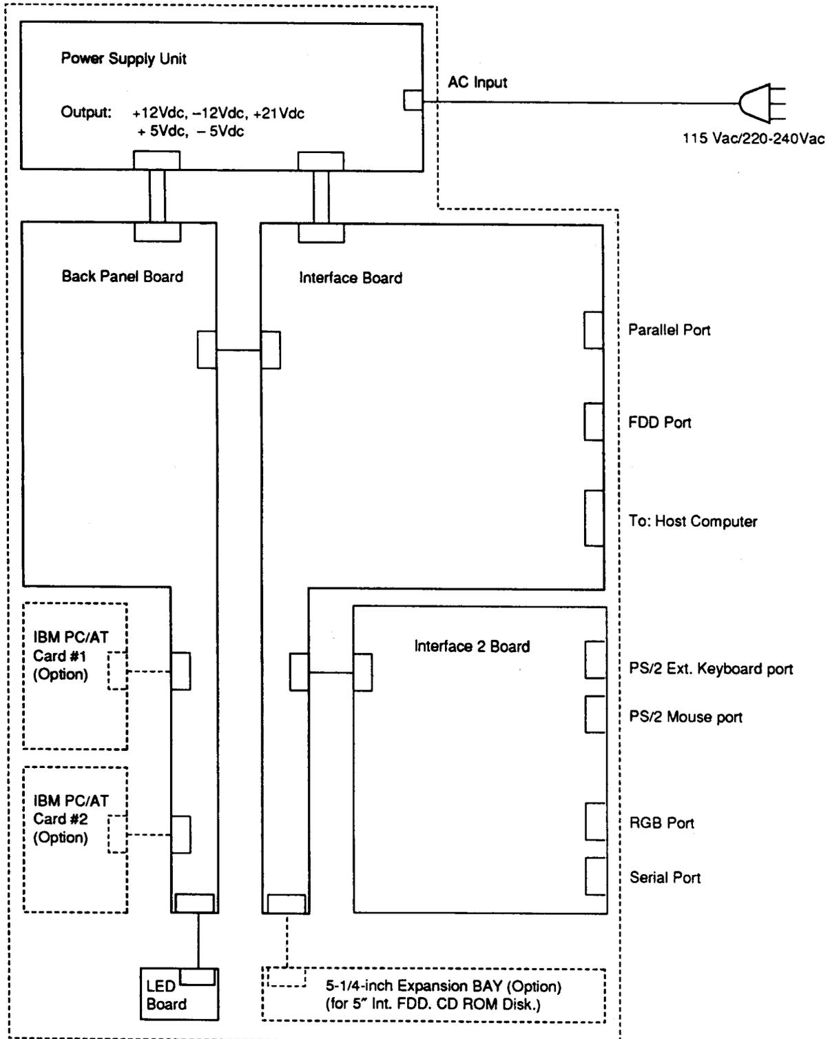
Figure 1-2 System Unit Block Diagram
