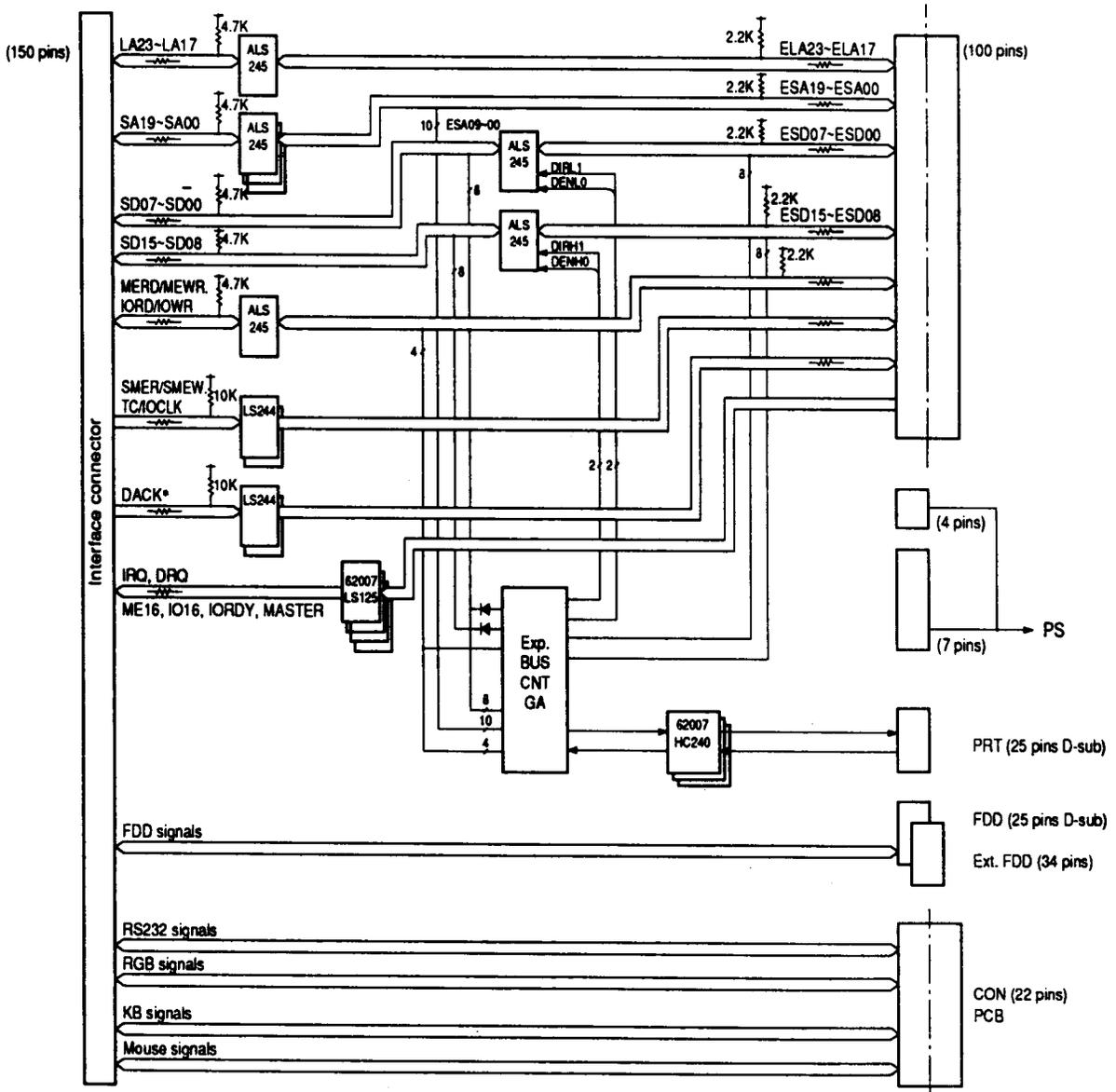
Figure 1-3 Interface Board Block Diagram
