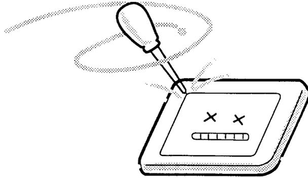
10. If you transport the module, do not use packing material that contains epoxy resin (amine) or silicon glue (alcohol or oxime). These materials can release gas that can damage the panel's polarization.
