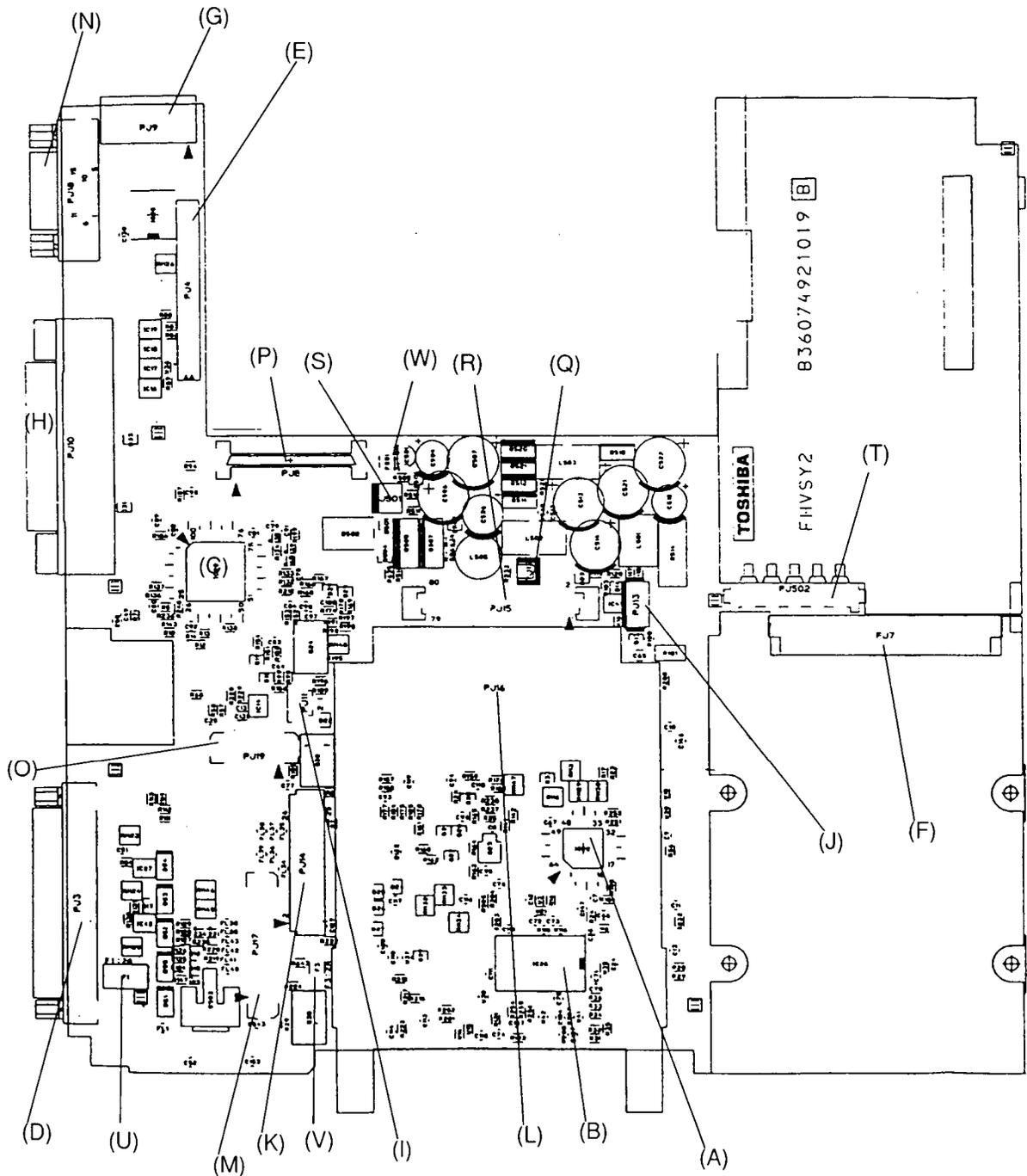
Figure B-1 FHVSY\* system board (front)
