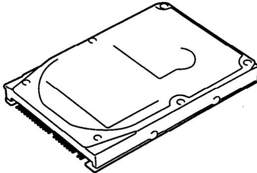
*Figure 1-4 2.5-Inch HDD*
