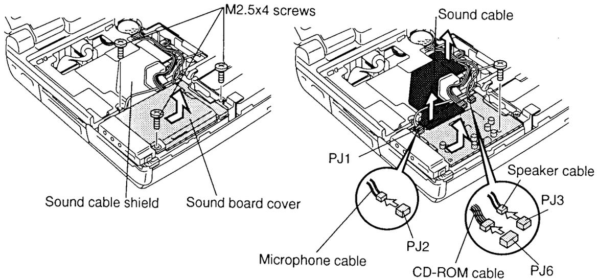
*Figure 4-13 Removing the sound board*
