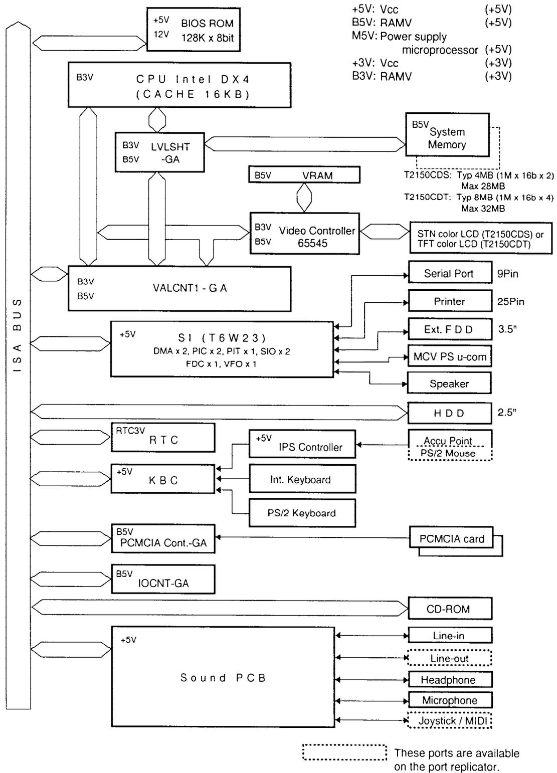
Figure 1-2 T2150 series system board block diagram
