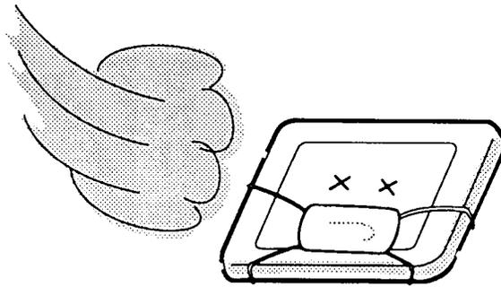
11. The TAB IC on the LCD back panel is easily damaged so be very careful when handling it.
