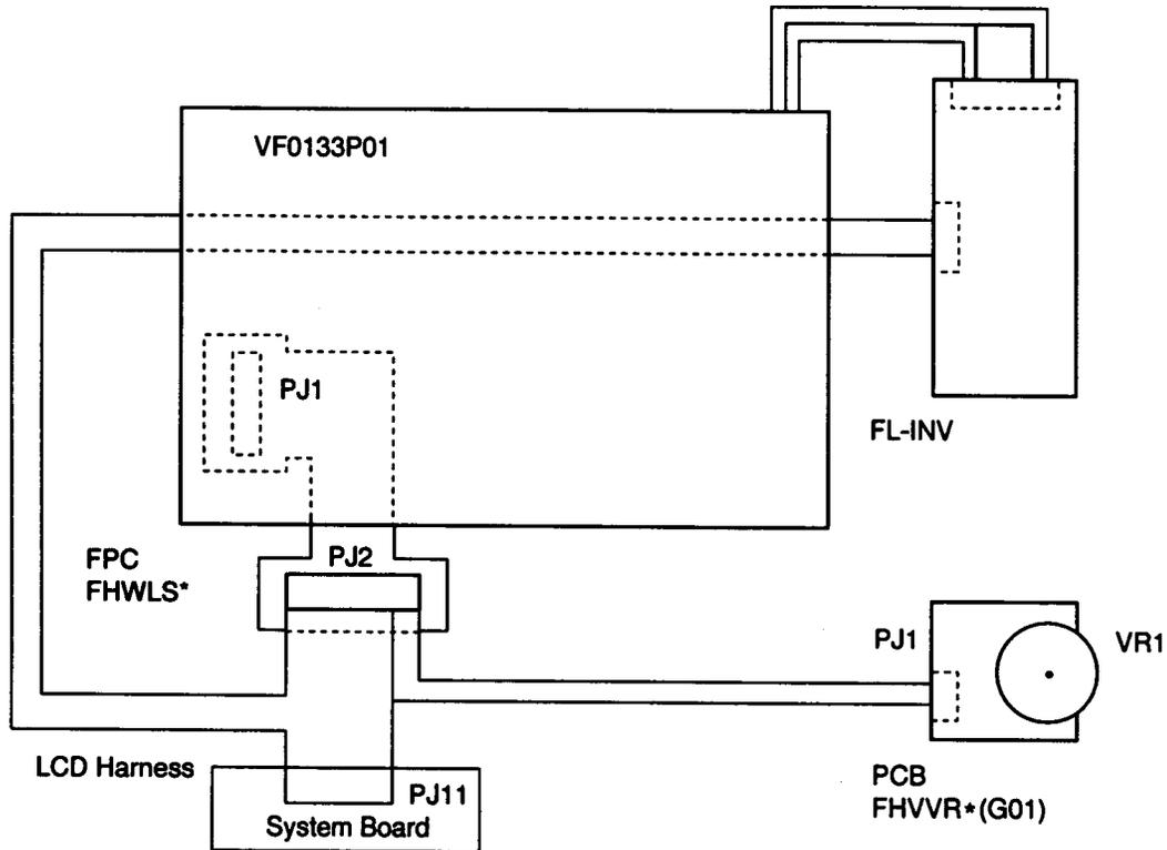
Figure 2-3 T2150CDS display connection
