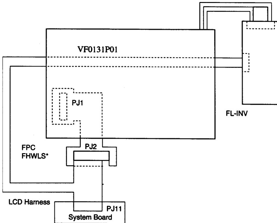
*Figure 2-4 T2150CDT display connection*
