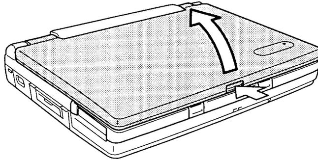
*Figure 4-1 Opening the display panel*
