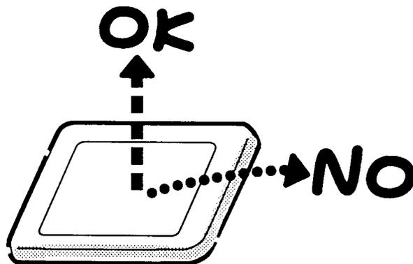
2. Be careful to align the holes at the four corners of the LCD module with the corresponding holes in the LCD cover before securing the module with screws. Do not force the module into place, because stress can affect its performance.
