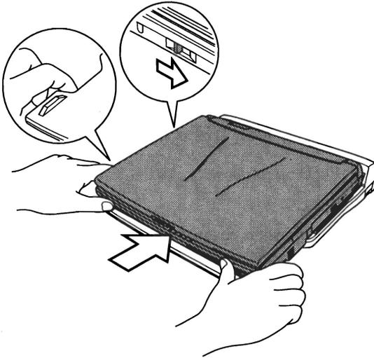
*Figure 8-25 Connecting to the Port Replicator*
