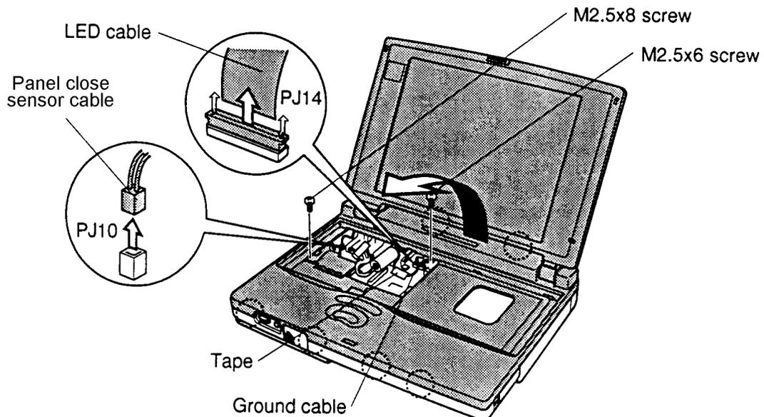
Figure 4-29 Removing the top cover with display assembly
