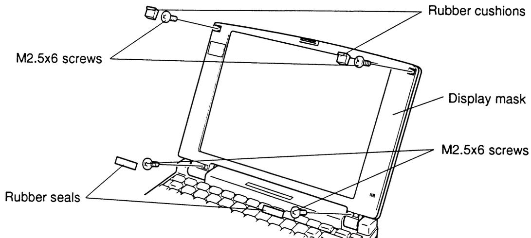
*Figure 4-41 Removing the rubber seals, cushions, and screws*
