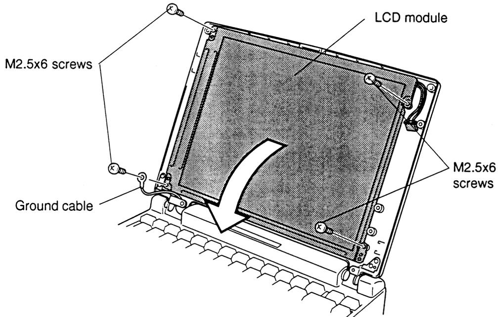
Figure 4-45 Removing the LCD module screws (TFT)
