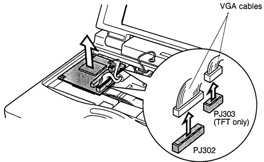
*Figure 4-25 Disconnecting the cables from the VGA board*
