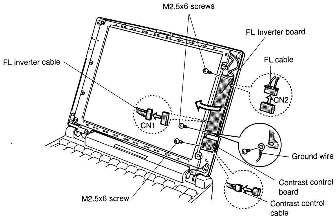
Figure 4-44 Removing the FL inverter board (DSTN)
