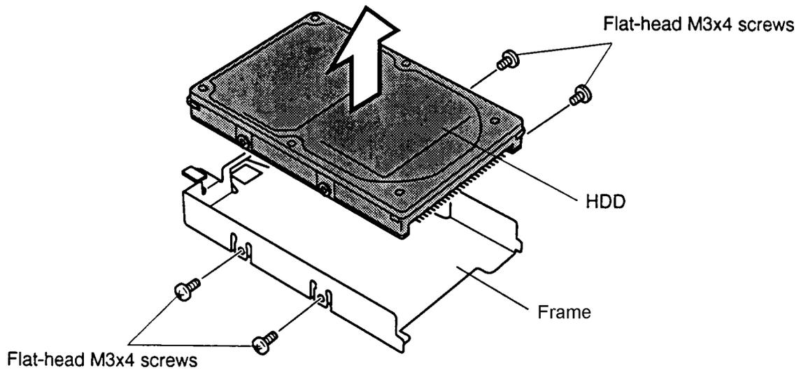
*Figure 4-17 Removing the HDD from the frame*
