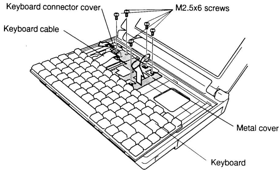
*Figure 4-19 Removing the metal cover*
