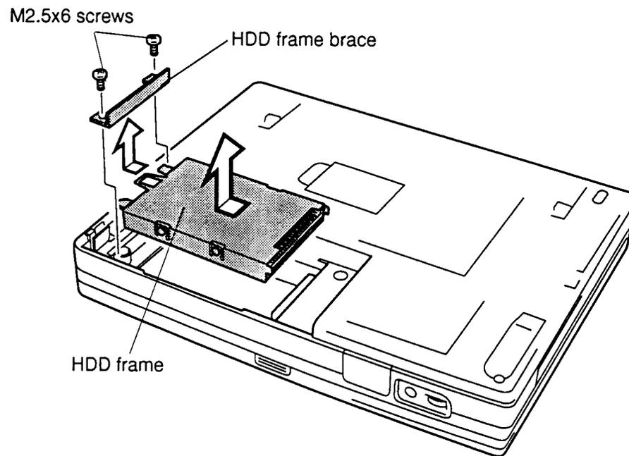
*Figure 4-16 Removing the frame with the HDD*
