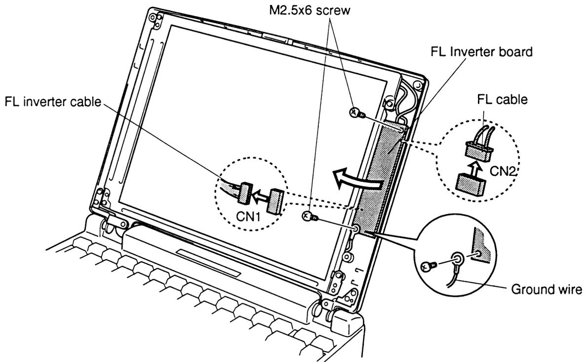
Figure 4-43 Removing the FL inverter board (TFT)
