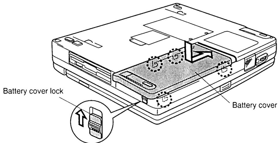
Figure 4-3 Installing the battery pack cover
