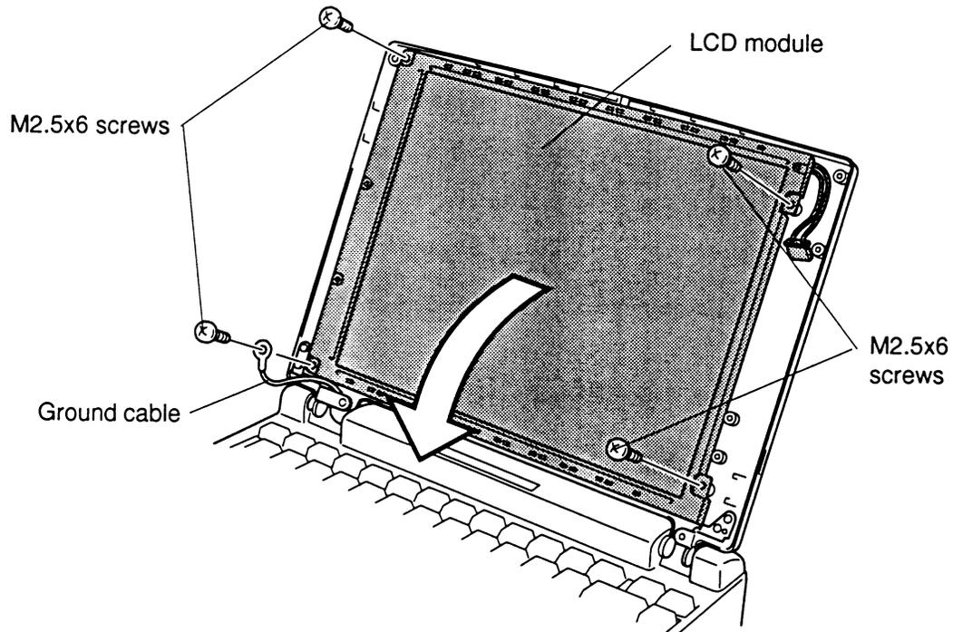
Figure 4-47 Removing the LCD module screws (DSTN)
