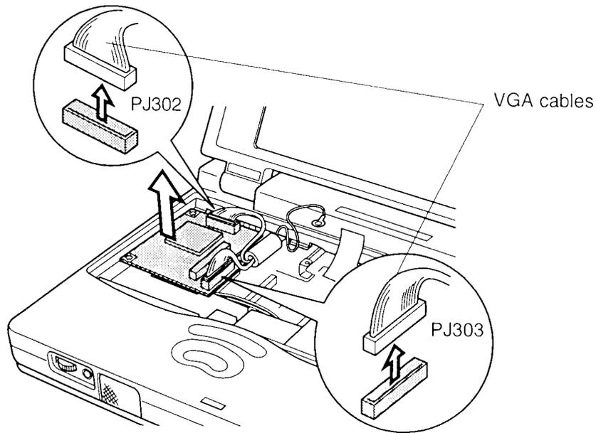
*Figure 4-24 Disconnecting the cables from the VGA board*
