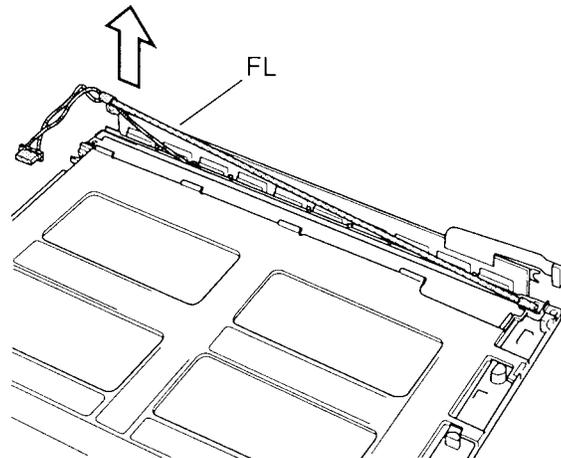
*Figure 4-43 Removing the DSTN FL*
