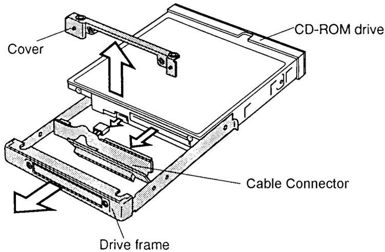
Figure 4-15 Removing the CD-ROM
