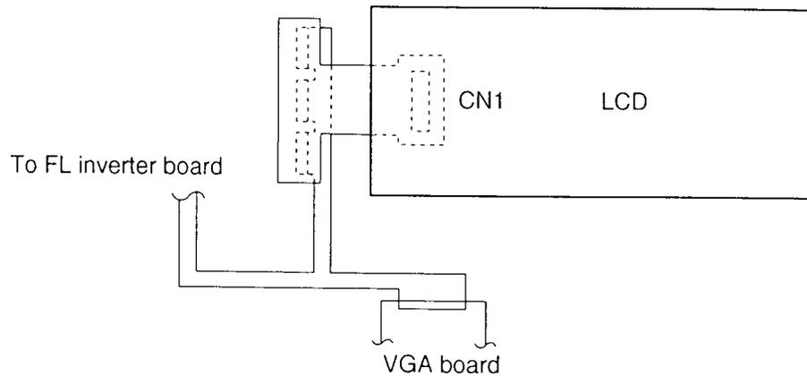
*Figure 2-4 410CDT display connection*
