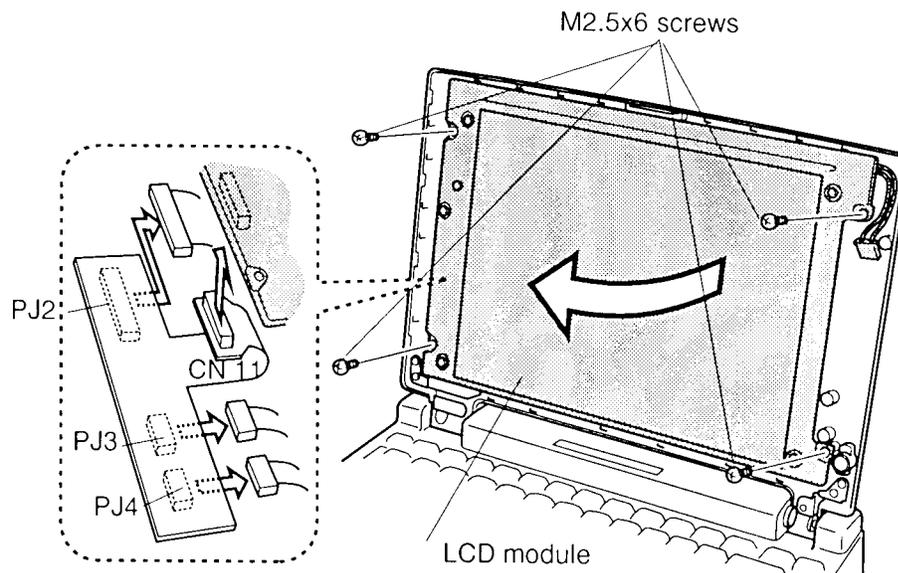
Figure 4-40 Removing the LCD module
