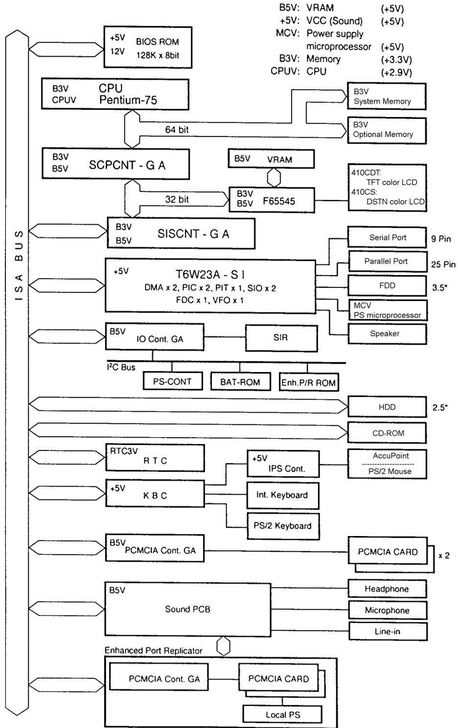
Figure 1-3 410 series system board block diagram
