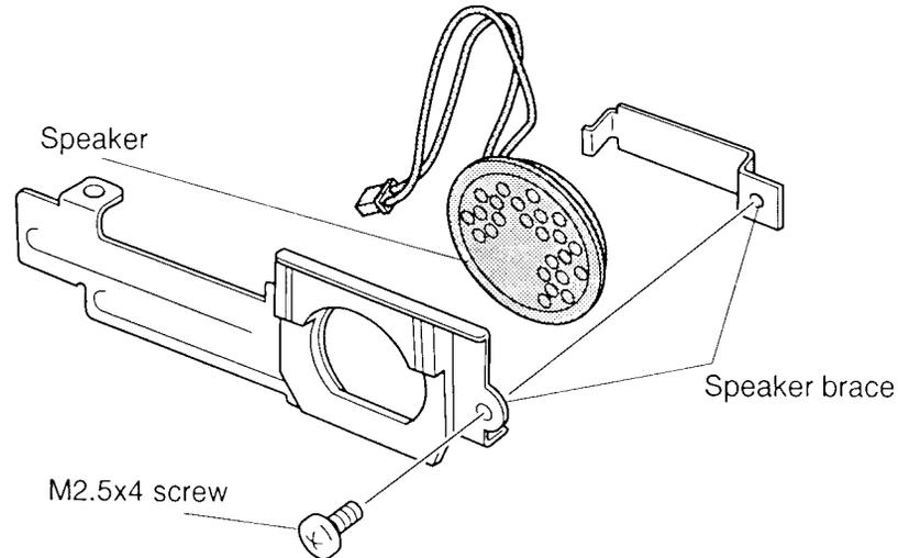
*Figure 4-34 Removing the speaker*
