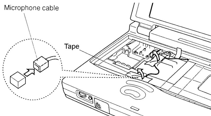
*Figure 4-22 Disconnecting the microphone cable*
