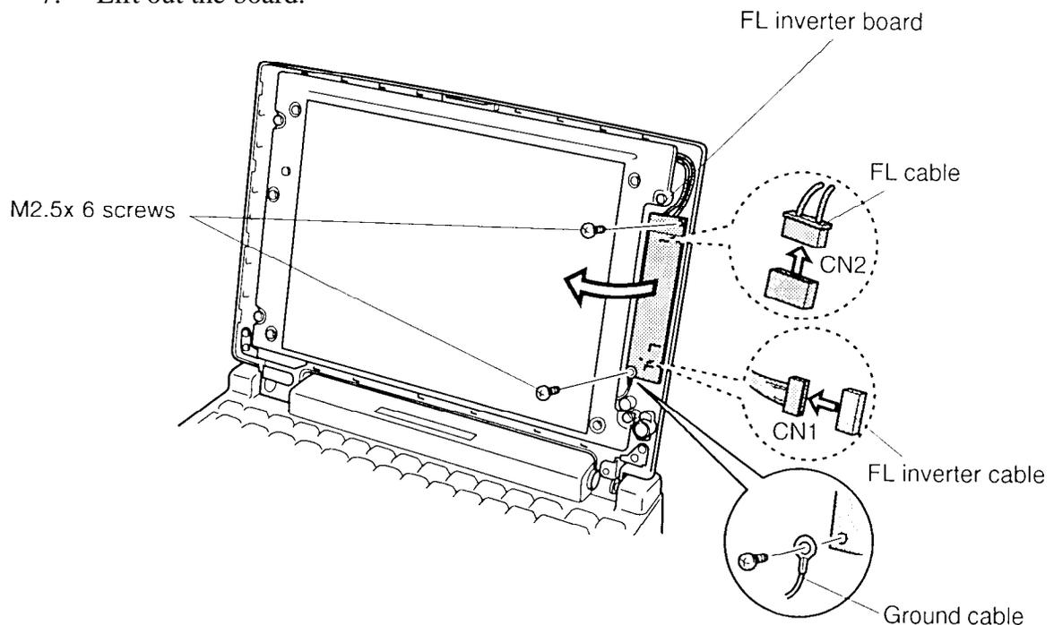
Figure 4-38 Removing the DSTN FL inverter board
