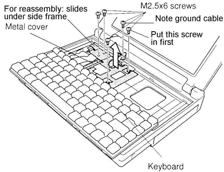
*Figure 4-19 Removing the metal cover*
