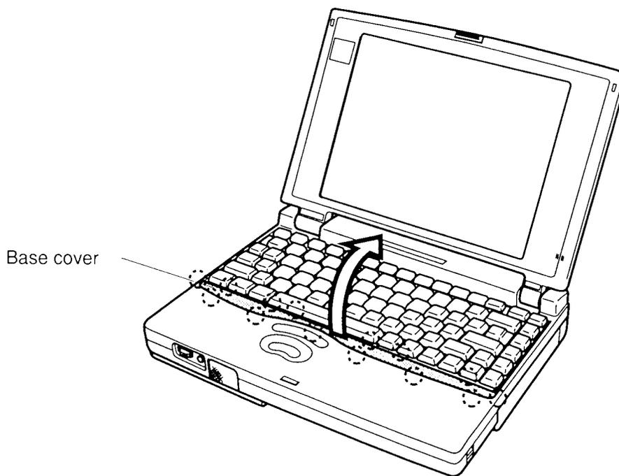
*Figure 4-18 Removing the keyboard base*
