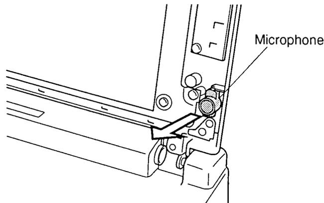
*Figure 4-45 Removing the microphone*
