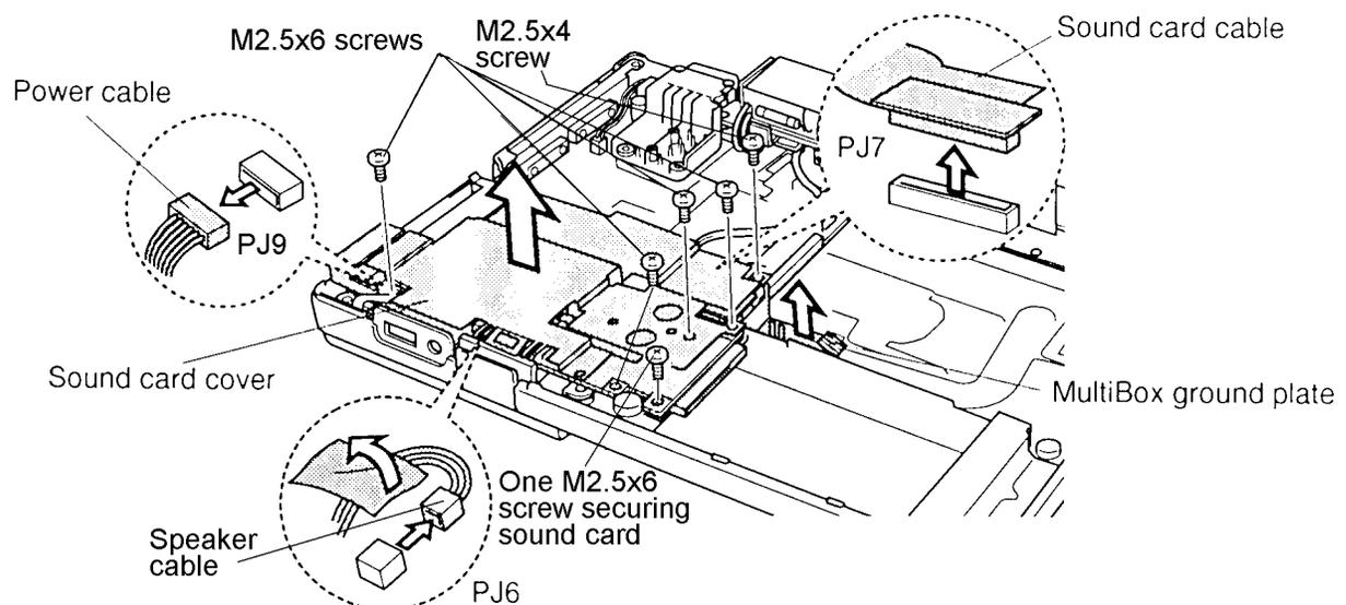
Figure 4-28 Removing the sound card
