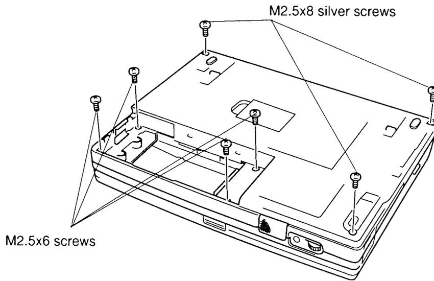
*Figure 4-25 Removing the top cover screws*
