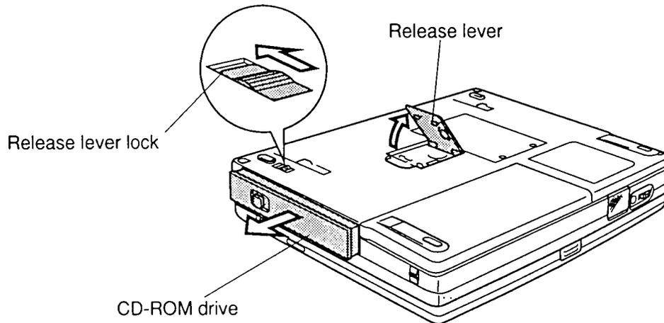
*Figure 4-13 Removing the CD-ROM drive*
