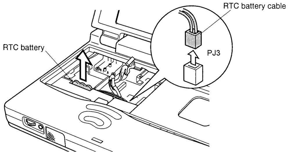
*Figure 4-26 Removing the RTC battery*
