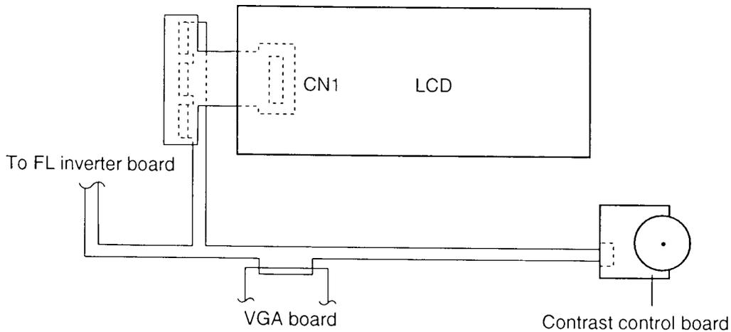
*Figure 2-3 410CS display connection*
