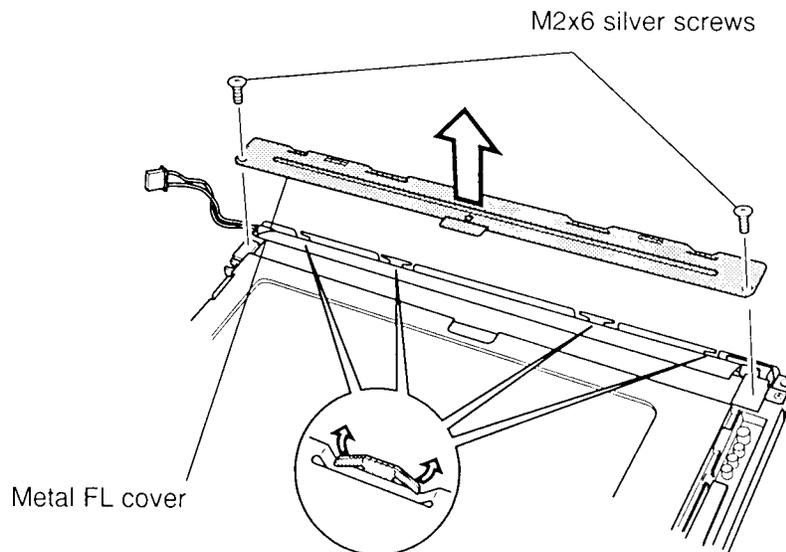
Figure 4-44 Removing the TFT FL
