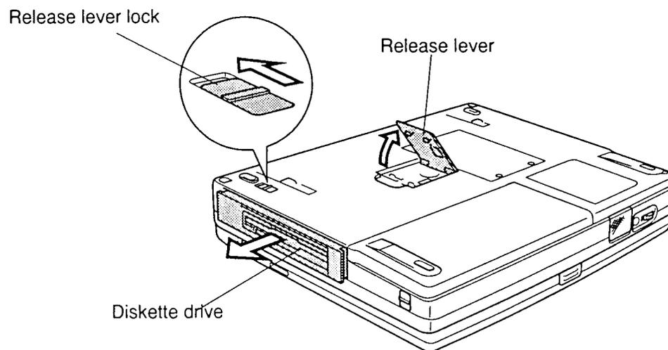
*Figure 4-9 Removing the diskette drive*
