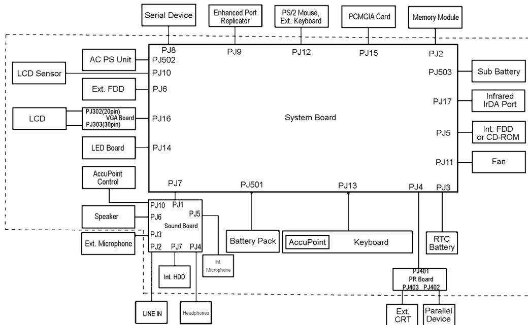
Figure 1-2 410 system unit configuration
