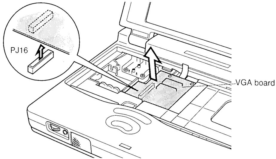
*Figure 4-23 Removing the VGA board*
