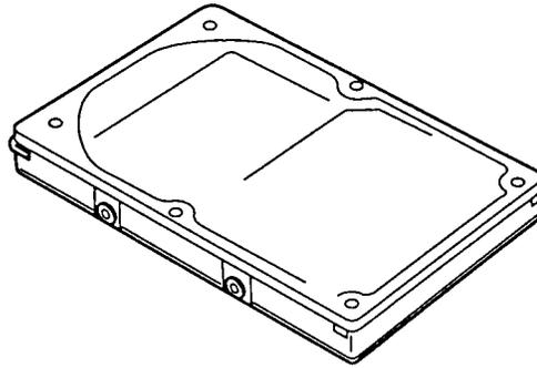
*Figure 1-5 2.5inch HDD*
