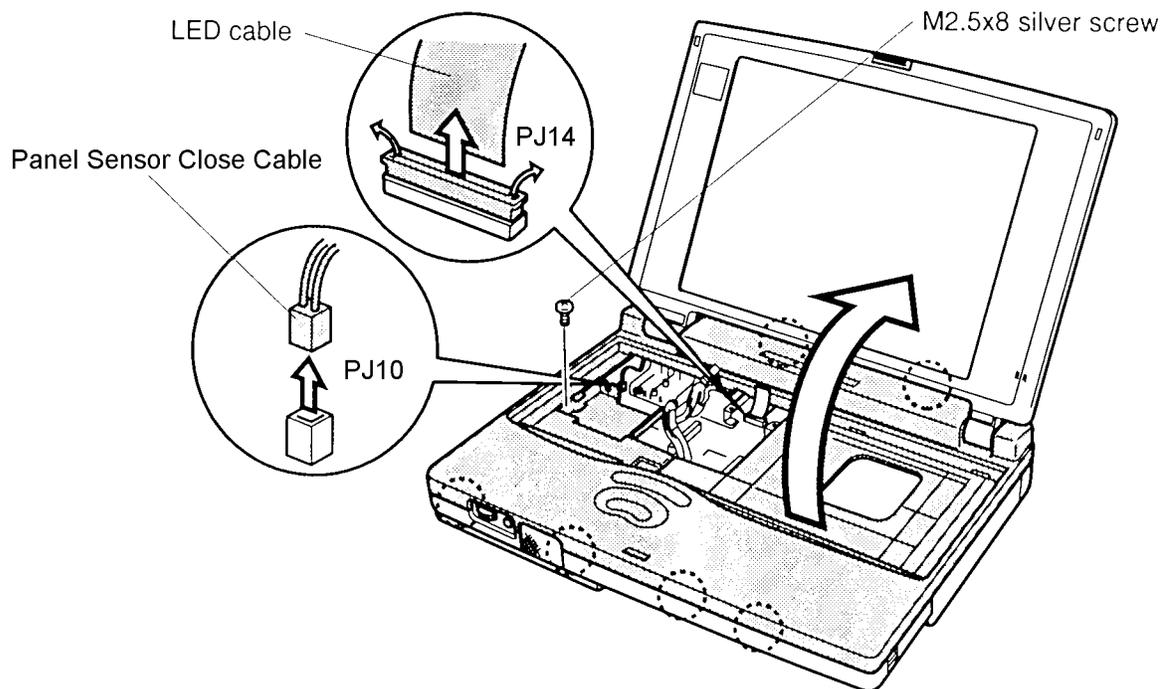
*Figure 4-27 Removing the top cover and display assembly*
