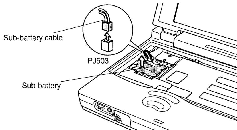
*Figure 4-21 Removing the sub-battery*
