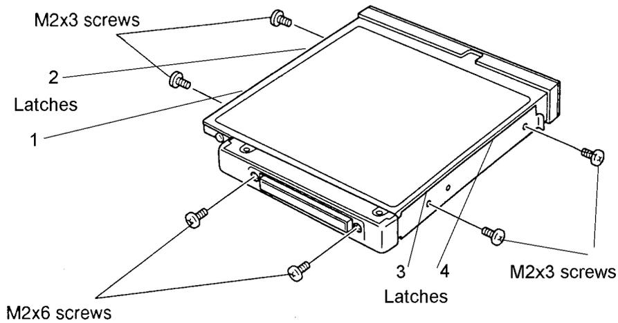
Figure 4-14 Removing the screws
