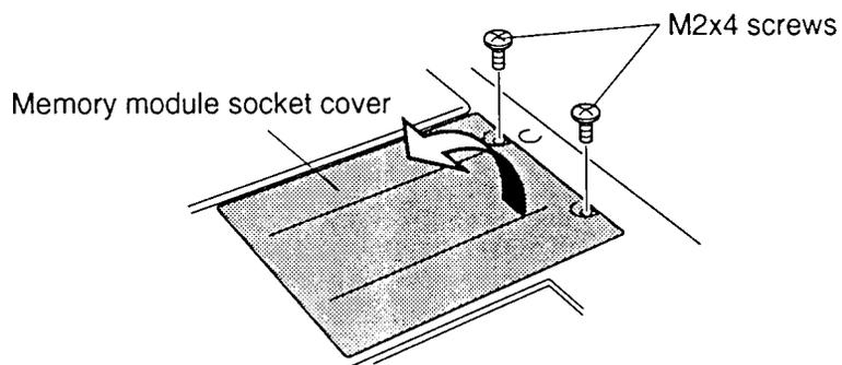
Figure 4-6 Removing the memory module socket cover
