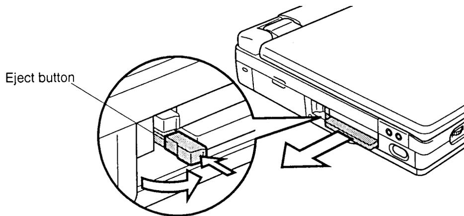
*Figure 4-4 Removing the PCMCIA card*
