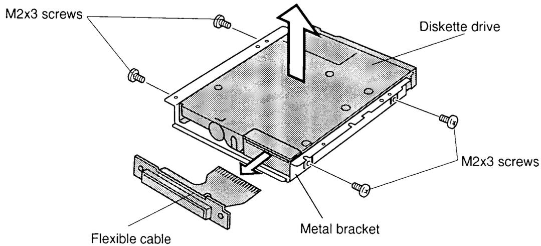
*Figure 4-12 Removing the diskette drive*
