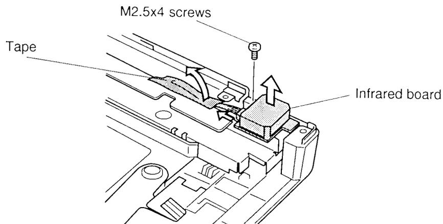
*Figure 4-32 Removing the infrared board*
