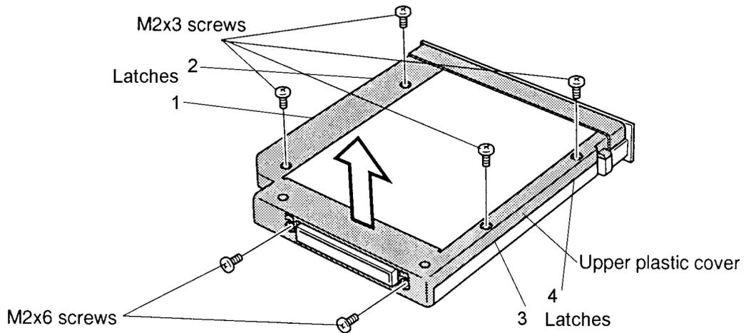
*Figure 4-10 Removing the screws*
