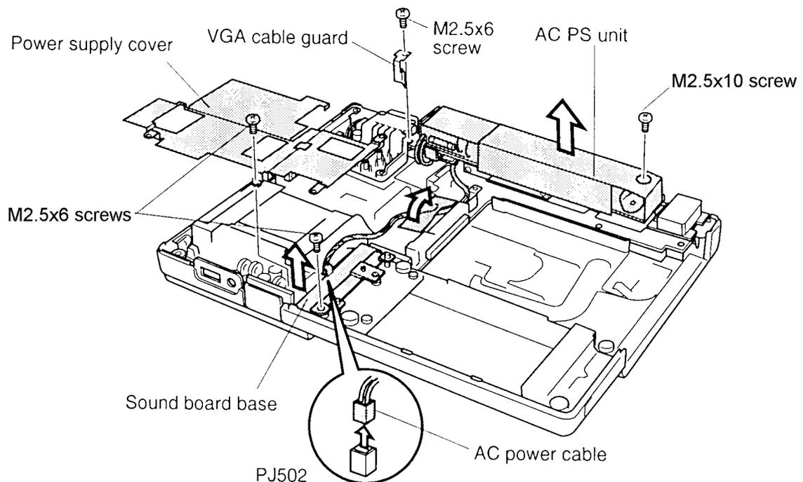
Figure 4-30 Removing the AC PS unit
