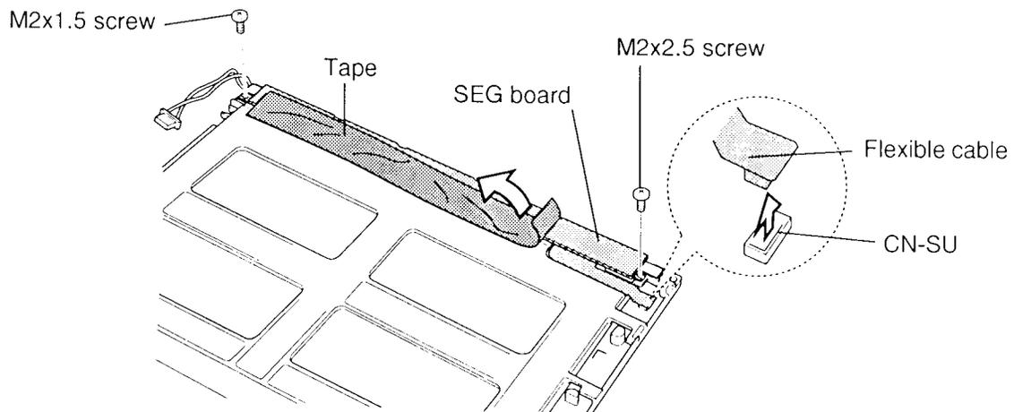
*Figure 4-41 Disconnecting the SEG board*
