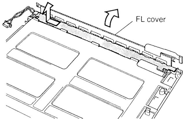
*Figure 4-42 Removing the FL cover*
