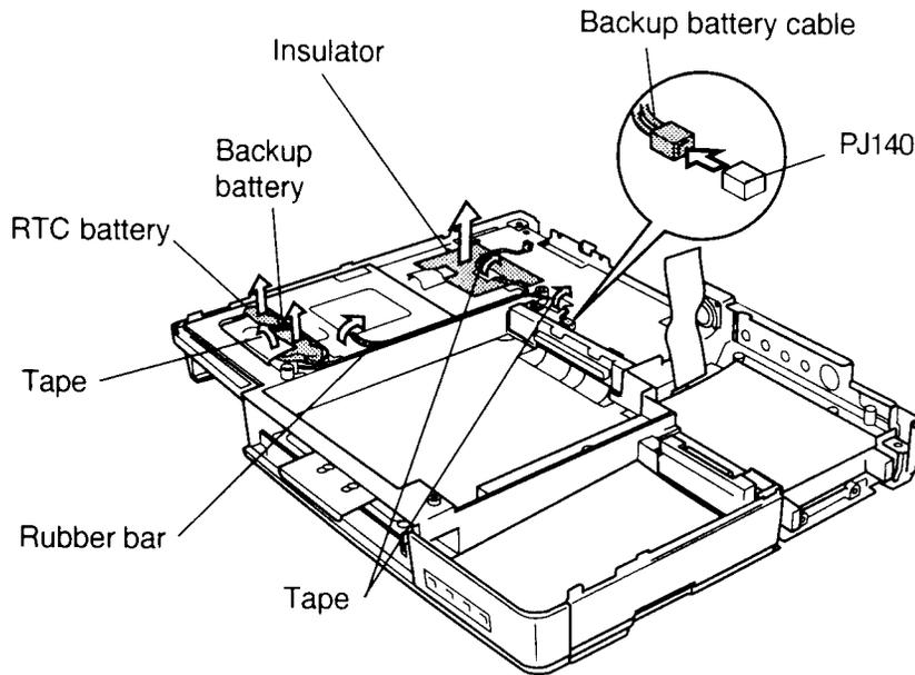
*Figure 4-35 Removing the RTC and backup batteries*
