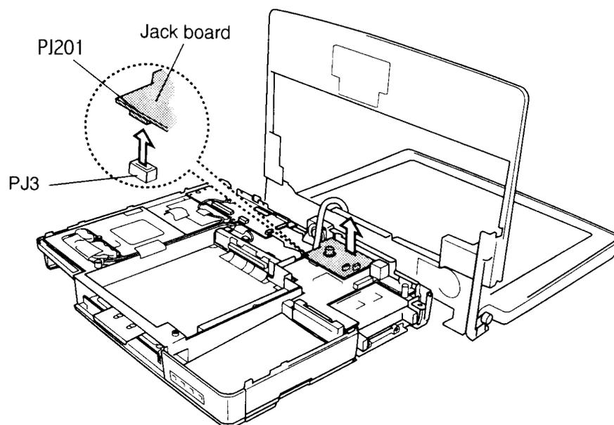
*Figure 4-31 Disconnecting the jack board*
