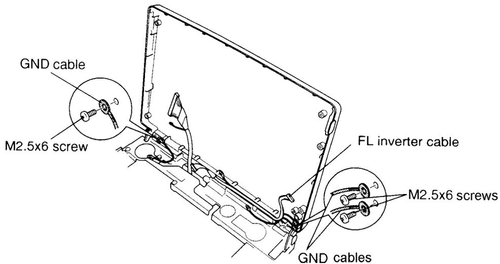
*Figure 4-47 Removing the ground cable screws*
