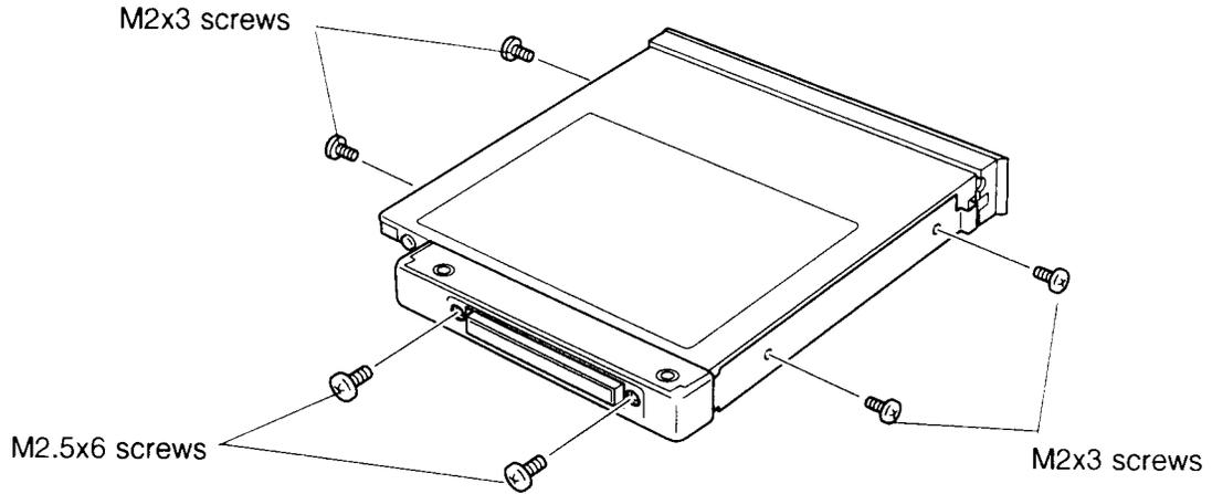
*Figure 4-12 Removing the CD-ROM screws*
