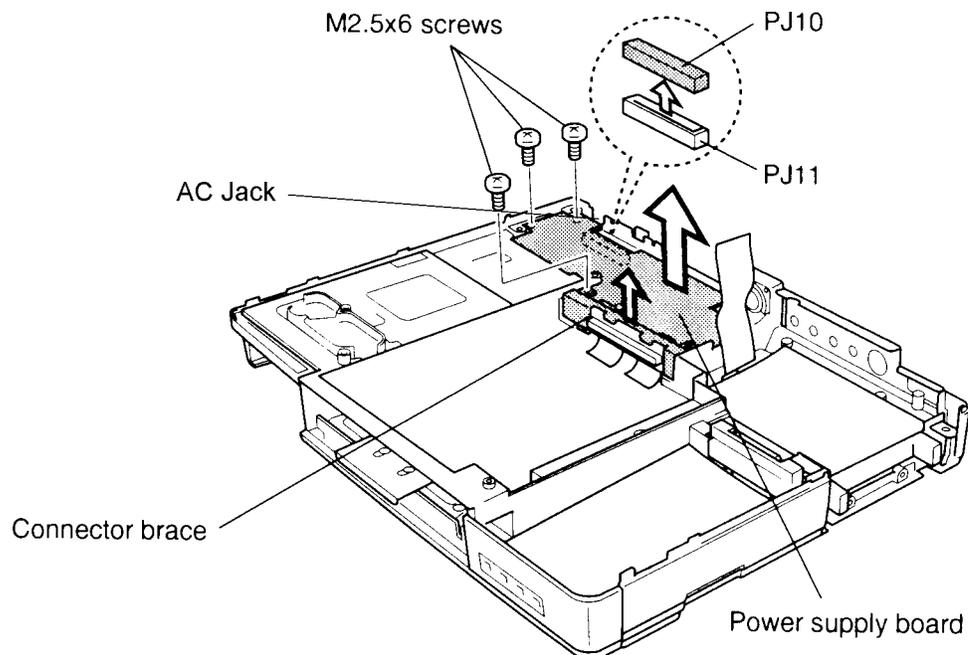
Figure 4-36 Removing the power supply board
