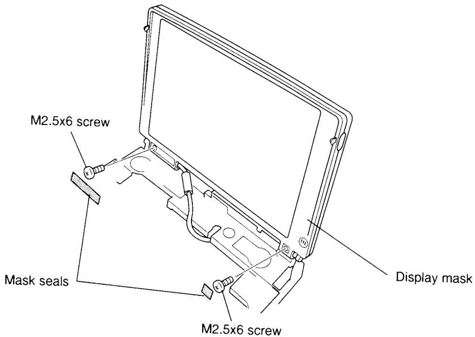
*Figure 4-43 Removing the display mask screws*
