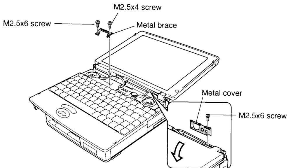
*Figure 4-20 Removing the metal brace and cover*
