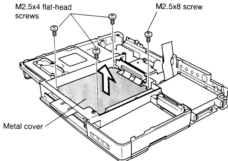
*Figure 4-37 Removing the metal cover*
