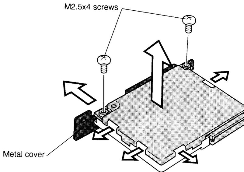
Figure 4-24 Removing the DAA module metal cover screws
