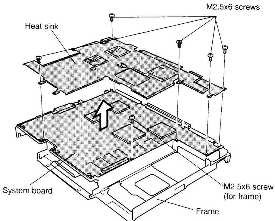
*Figure 4-41 Separating the system board, heat sink, and frame*
