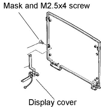
*Figure 4-49 Removing the display cover*
