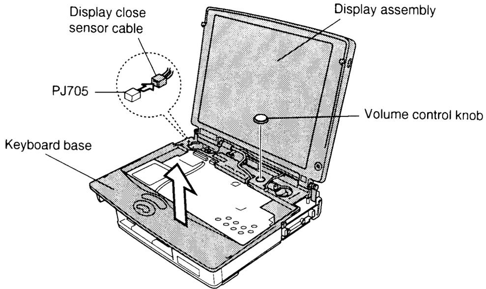
*Figure 4-28 Removing the volume control knob and lifting up the keyboard base*
