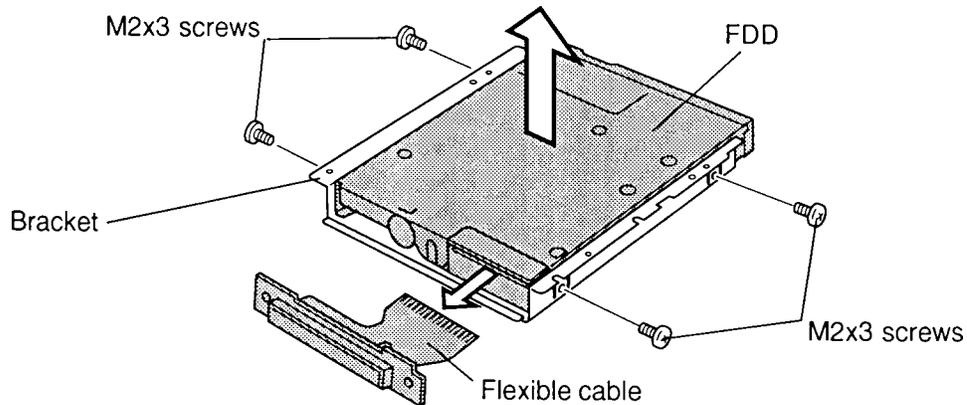
*Figure 4-9 Removing the FDD from the bracket*
