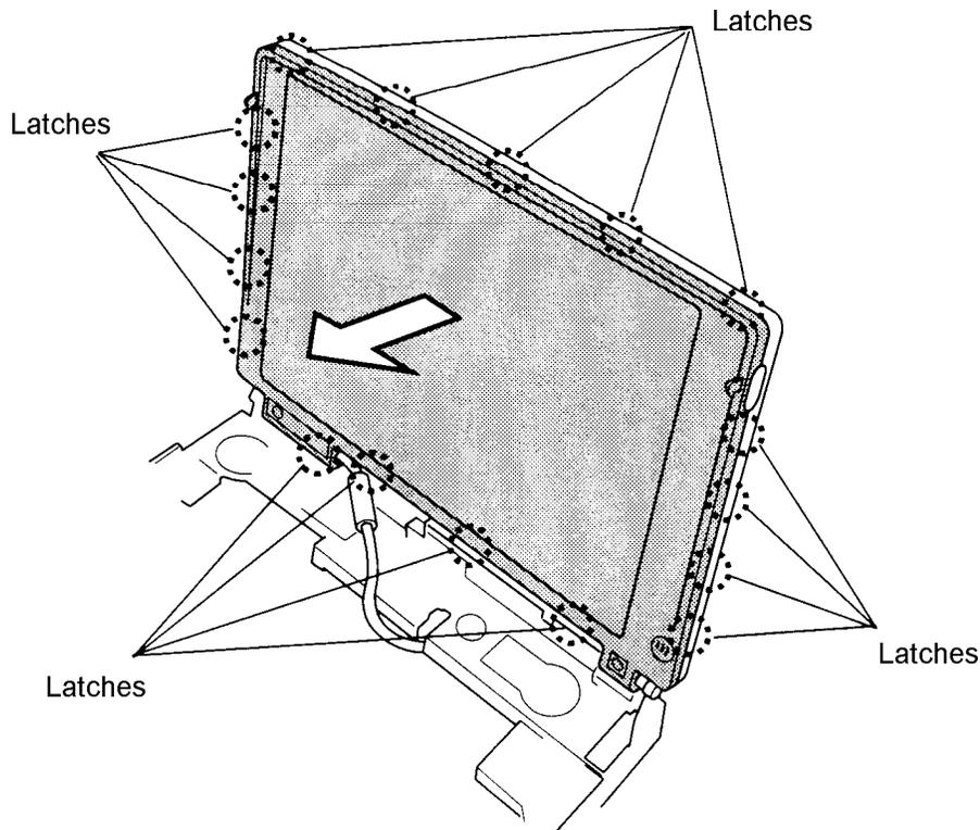
*Figure 4-44 Removing the display mask*
