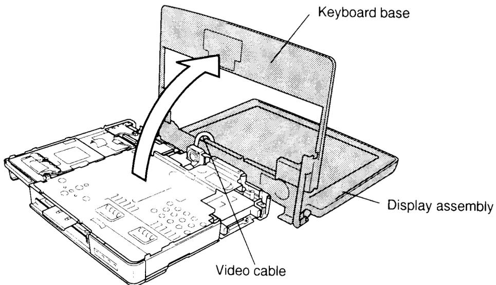
*Figure 4-29 Removing the keyboard base and display assembly*
