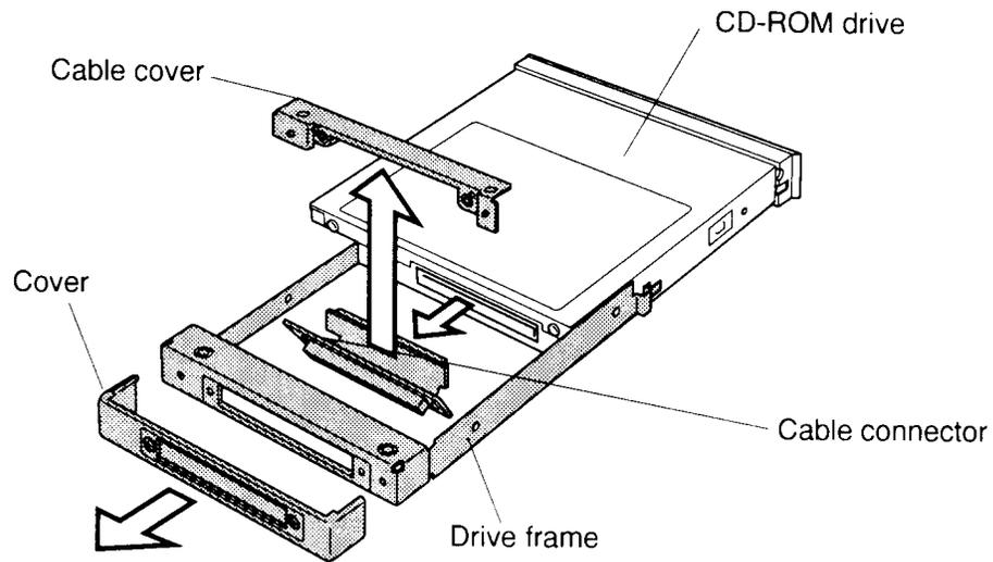
*Figure 4-13 Removing the CD-ROM*
