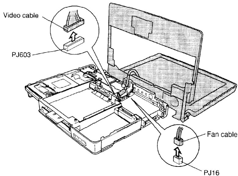
*Figure 4-33 Disconnecting the video cable and fan cable*
