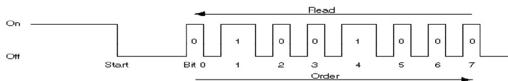
Check 1 Convert the DC IN icon blink pattern into the hexadecimal error code and compare it to the following tables.
