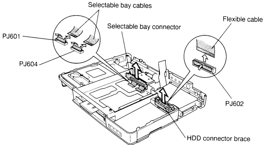
*Figure 4-38 Disconnecting the flexible cables*
