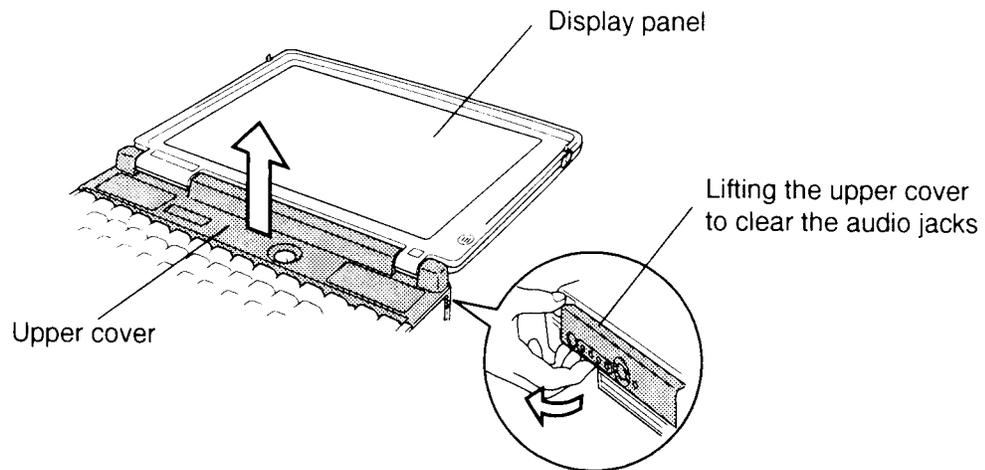
*Figure 4-19 Removing the upper cover*
