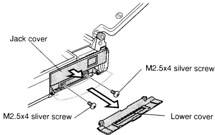
*Figure 4-22 Removing the lower cover screws*
