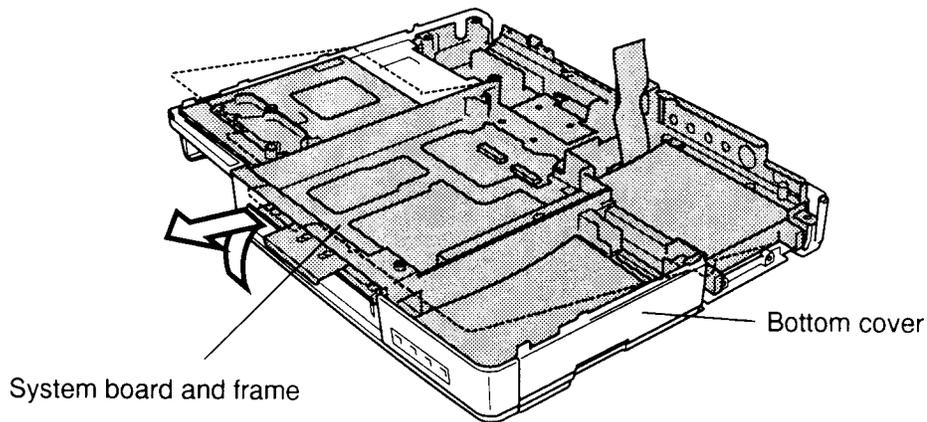
*Figure 4-40 Removing the frame and system board*
