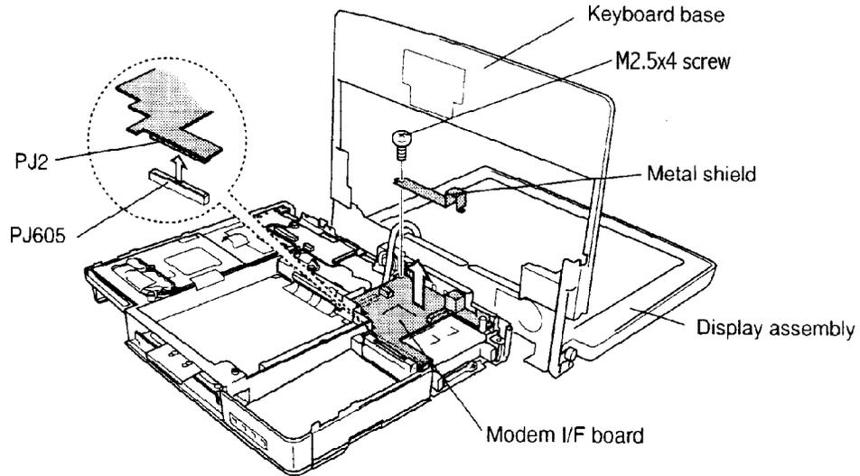
*Figure 4-32 Removing the modem board*
