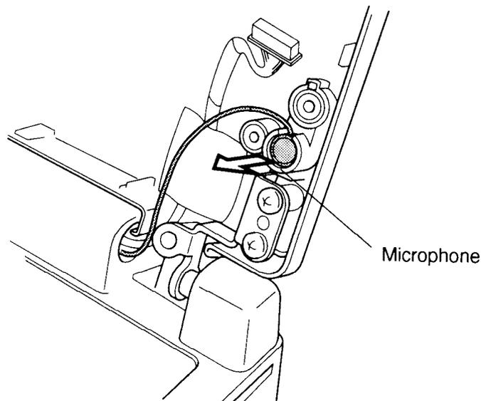
*Figure 4-48 Removing the microphone*
