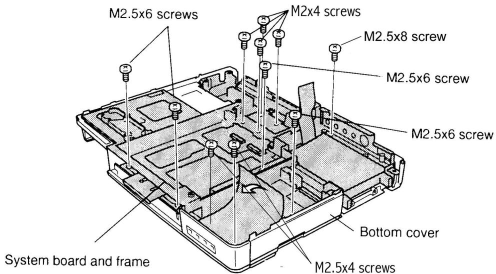
*Figure 4-39 Removing the frame and system board screws*
