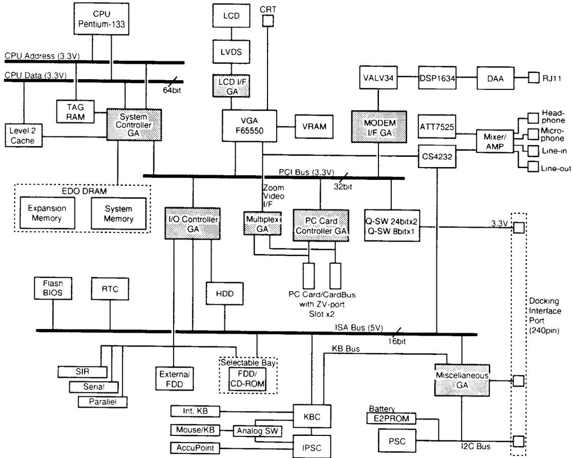
Figure 1-3 System board block diagram
