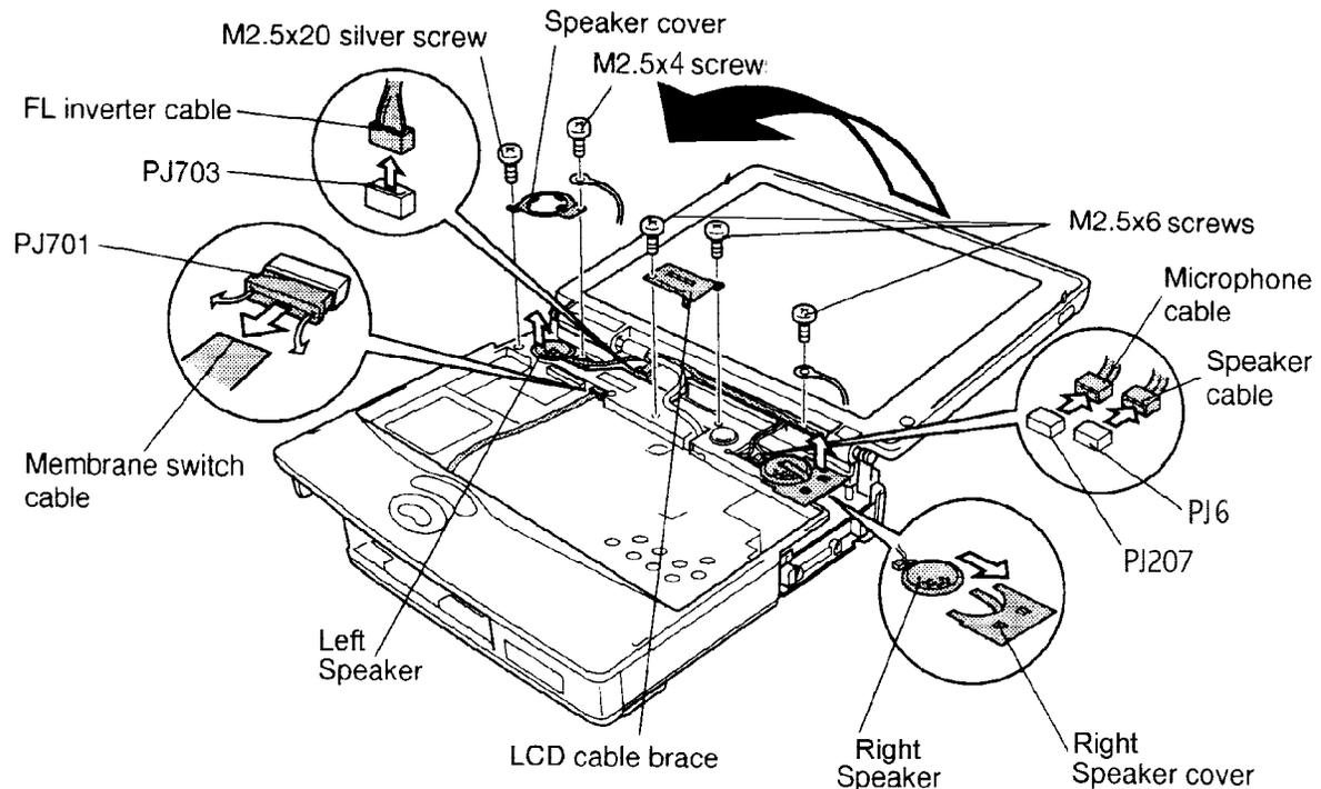
*Figure 4-27 Removing cables*
