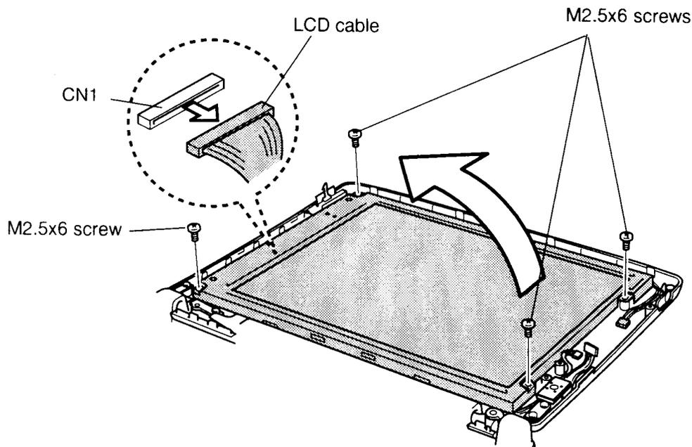
Figure 4-46 Removing the LCD module
