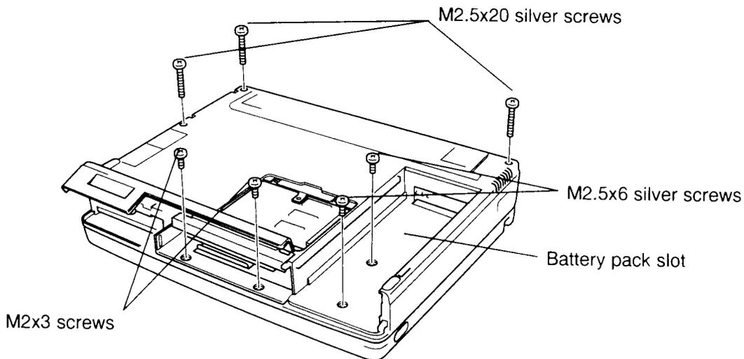
Figure 4-26 Removing the screws
