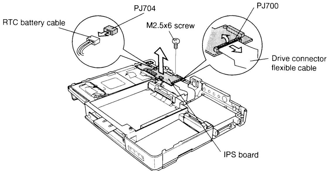
Figure 4-34 Removing the IPS board
