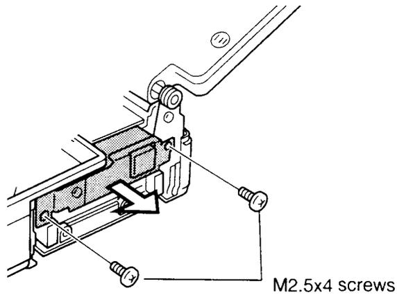
Figure 4-23 Removing the DAA module screws
