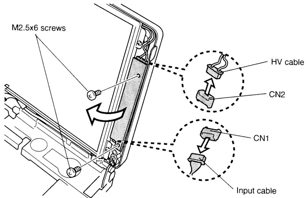
Figure 4-45 Removing the FL inverter board
