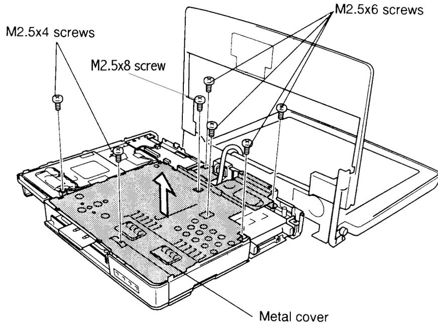
*Figure 4-30 Removing the metal cover*
