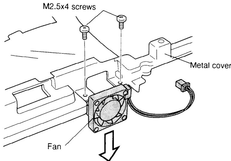
*Figure 4-42 Removing the fan*
