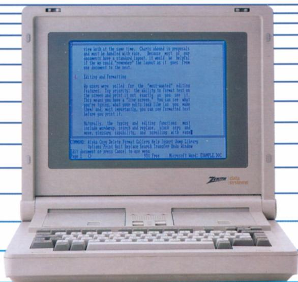
*The Z-181 boasts perhaps the most advanced screen available in a portable... display images are crisp, bold and bright. The Z-181 weighs less than 12 pounds, features large capacity 3½" drives, and runs IBM PC/XT compatible software.*
