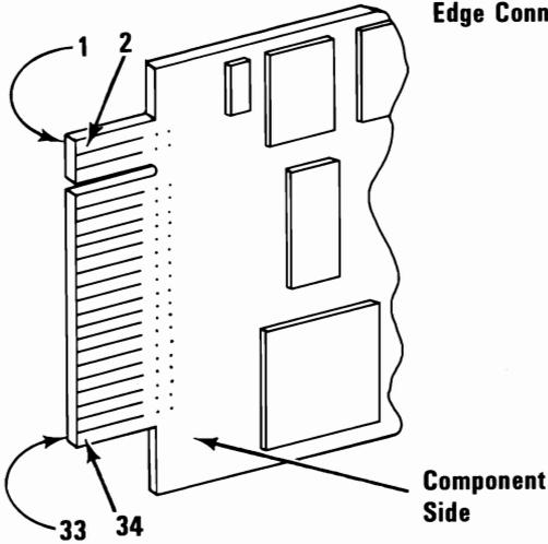
**Note:** Lands 1-33 (odd numbers) are on the back of the board. Lands 2-34 (even numbers) are on the front, or component side.
